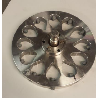
Figure 3.10 Sample holder on Struers Tegramin-25
