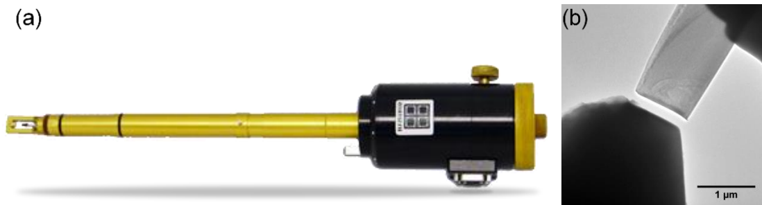
Figure 3.7 (a) The in-situ compression test holder - Hysitron PI95 TEM Pico-Indenter (b) TEM image of a pillar ready to be tested
