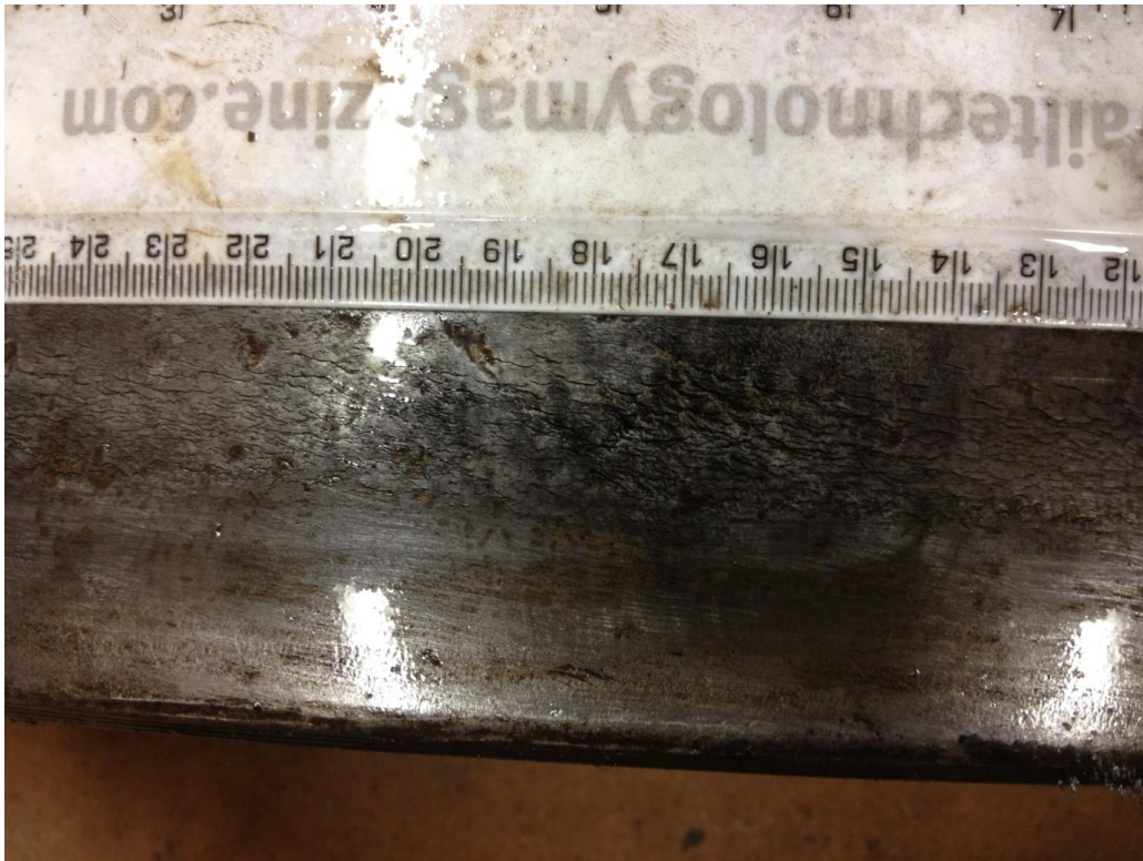
Figure 9.61 shows fine cracks found near the non-flange end of the HSR2 railway wheel and oriented approx. at 90^{\circ} to the circumference of the wheel tread surface and present across most of the entire circumferential length of the wheel at a position of 3 cm from the non-flange end.
