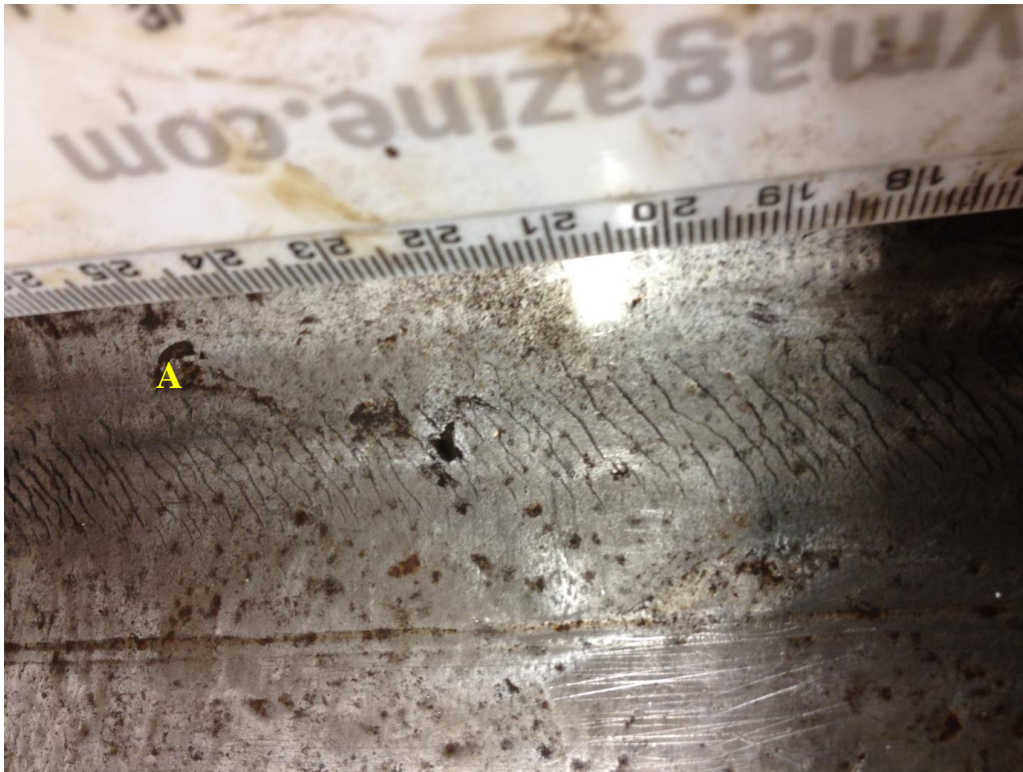
Figure 9.59 shows closely spaced and shallow cracks found near the flange of the HSR2 railway wheel and oriented approx. at 60^\circ to the circumference of the wheel tread surface and present across most of the entire circumferential length of the wheel.
