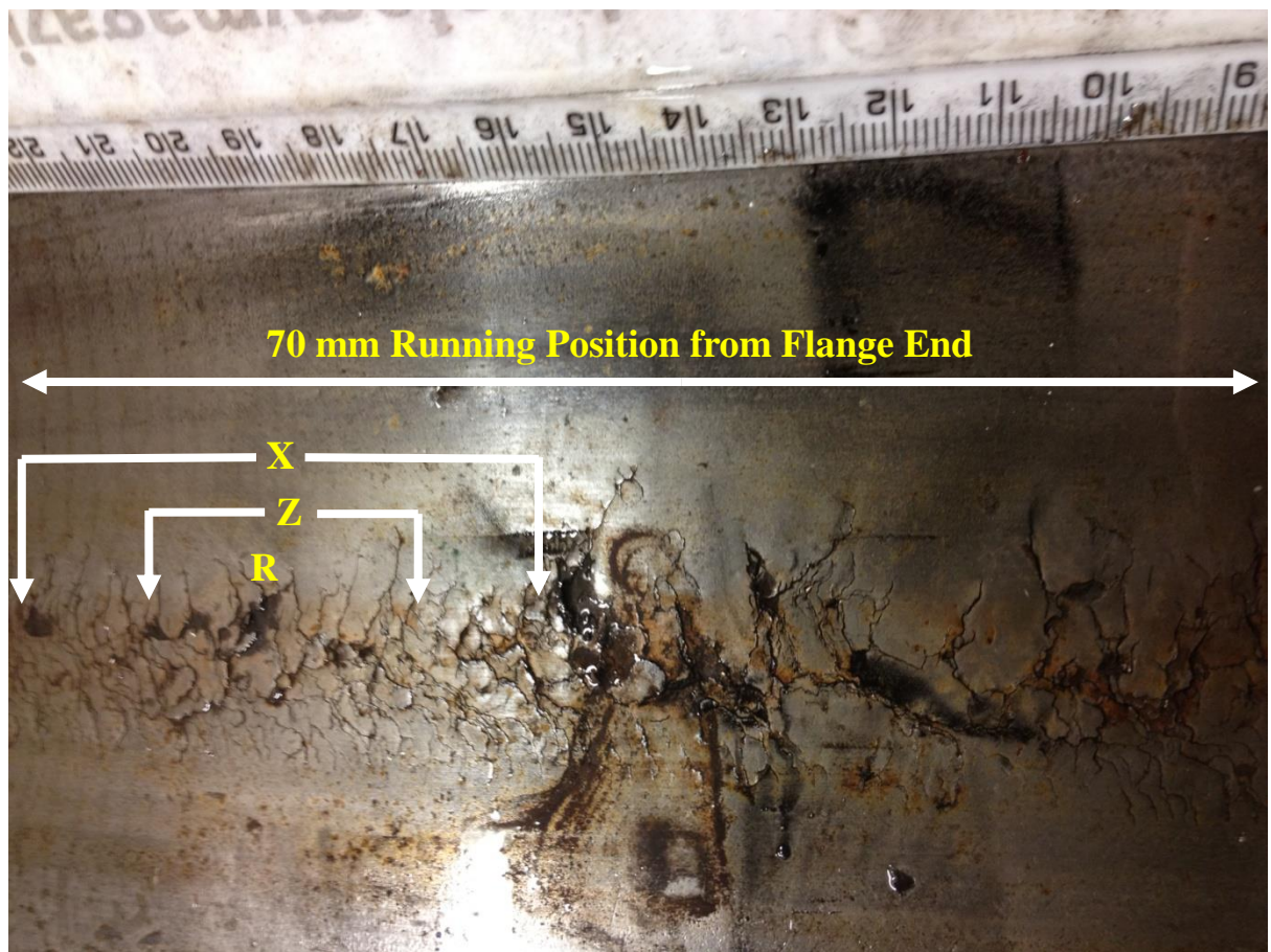
Figure 9.72 shows another image highlighting specific areas of the RCF prone region on the tread of wheel HSR1 showing the severe level of surface RCF damage that has occurred between 4 and 6 cm from the non-flange end of this wheel. Locations at which the subsequent ACFM scans (figures 9.71-9.73 incl. below) conduct+ed on this wheel tread have been clearly labelled on the photograph. Note that this figure is shown as figure 7.33 in chapter 7 of the PhD thesis above and has been reproduced here to keep it in context as it is part of this report and for the ease of the reader.
