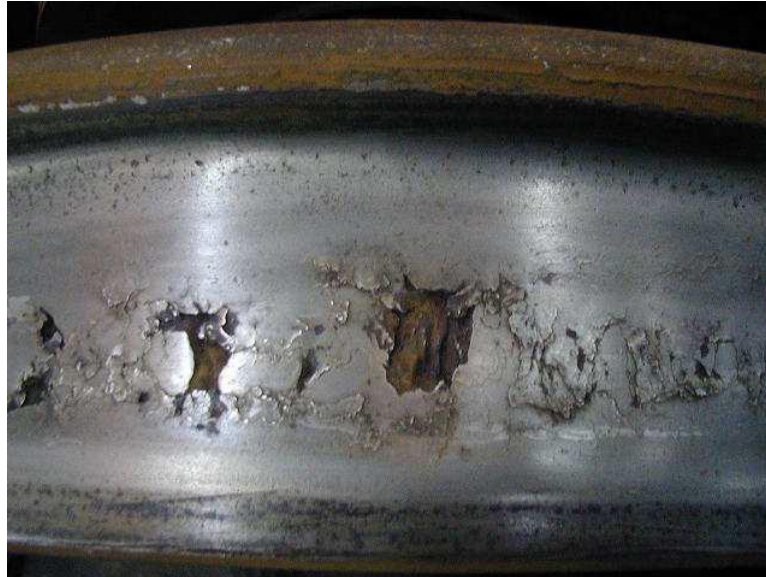
Figure 3.2 shows the presence of shelling and cavities on the wheel tread surface (the original of the above photographic image is shown in reference [11] and has been reproduced and appropriately referenced here for the purpose of this PhD thesis).
