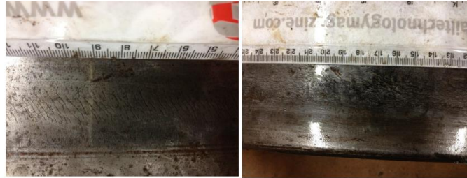
Figure 6.5 high magnification photographs of the HSR2 railway wheel tread surface showing the two circumferential band of RCF cracks: first band consists of shallow and fine cracks oriented at approx. 60^{\circ} to the circumferential direction of the tread found near the flange and the second circumferential band of cracks are oriented almost perpendicular ( 90^{\circ} \pm 0.5^{\circ} ) to the circumferential direction of the tread and are found at approx. 3 cm from the non-flange end of the tread. These two bands of RCF cracks are regions of interest for the 3-D reconstruction of cracks using the multi-sectioning in conjunction with optical metallography approach and ACFM scans across these cracks as presented in chapters 4 and 6, respectively.
