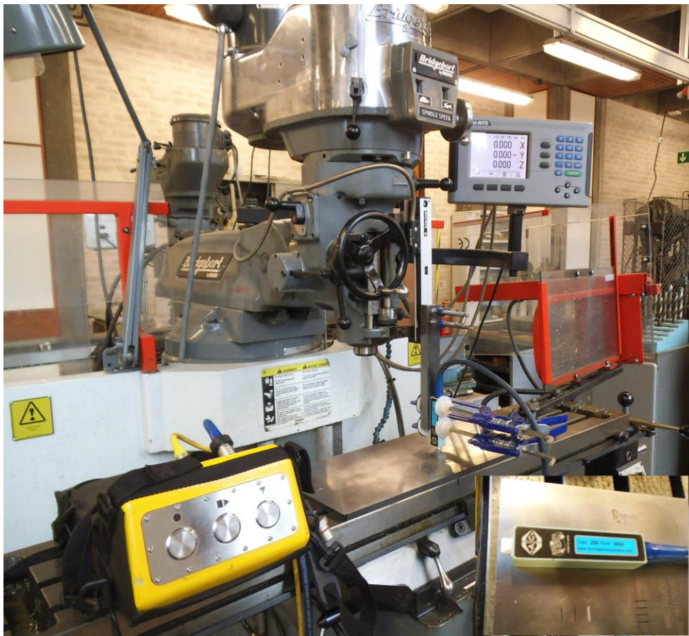
Figure 7.5 a digital photograph showing the ACFM system in the bottom left hand corner of the above image together with the probe (inset in the bottom right hand corner of the image).
