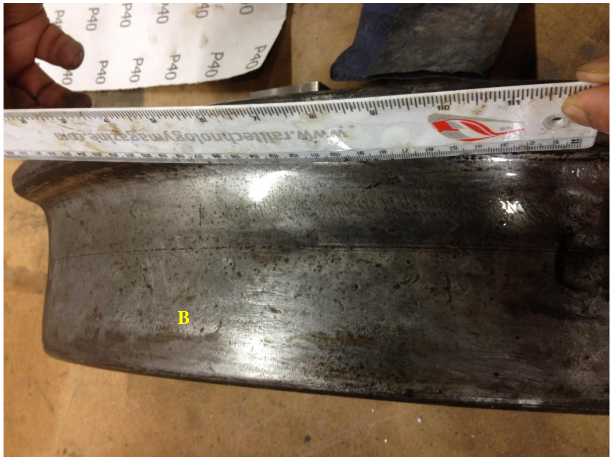
Figure 9.62 Feature B on railway wheel HSR2 scanned by ACFM.
