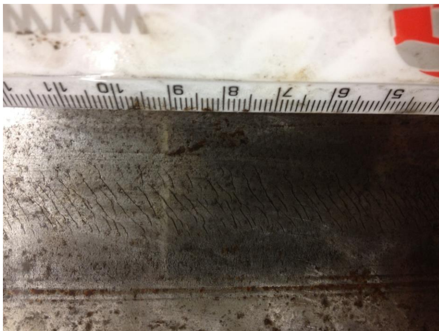
Figure 9.56 Fine cracks found near the flange end and across most of the entire circumferential length of the HSR2 railway wheel at a position of 9.0 cm from the non-flange end.
