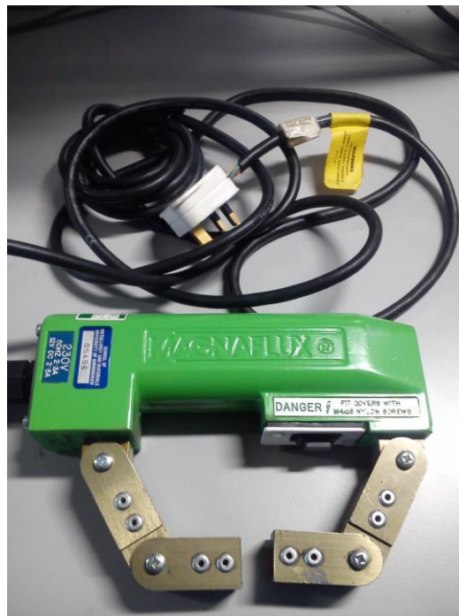
Figure 7.7 a digital photograph showing the magnetic particle inspection (MPI) system.
