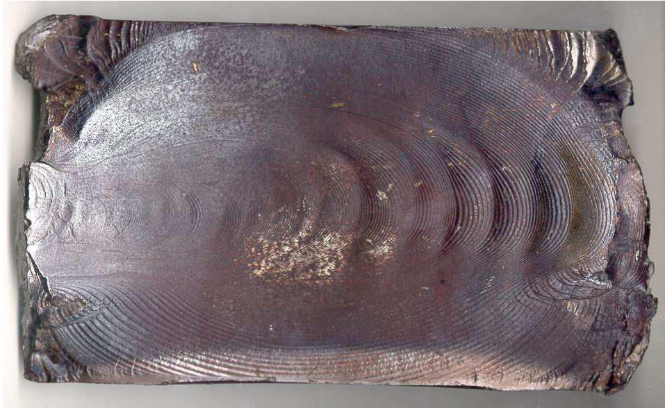
Figure 3.8 shows deep sub-surface tread defect (the original of the above photographic image is shown in reference [11] and has been reproduced and appropriately referenced here for the purpose of this PhD thesis).
