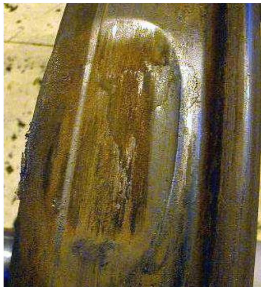
Figure 3.4 shows a wheel flat (the original of the above photographic image is shown in reference [11] and has been reproduced and appropriately referenced here for the purpose of this PhD thesis).
