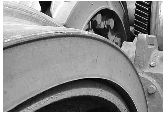
Figure 3.7 shows a schematic and a photograph of wheel tread roll-over (the originals of the above schematic and photographic image are shown in reference [11] and have been reproduced and appropriately referenced here for the purpose of this PhD thesis).
