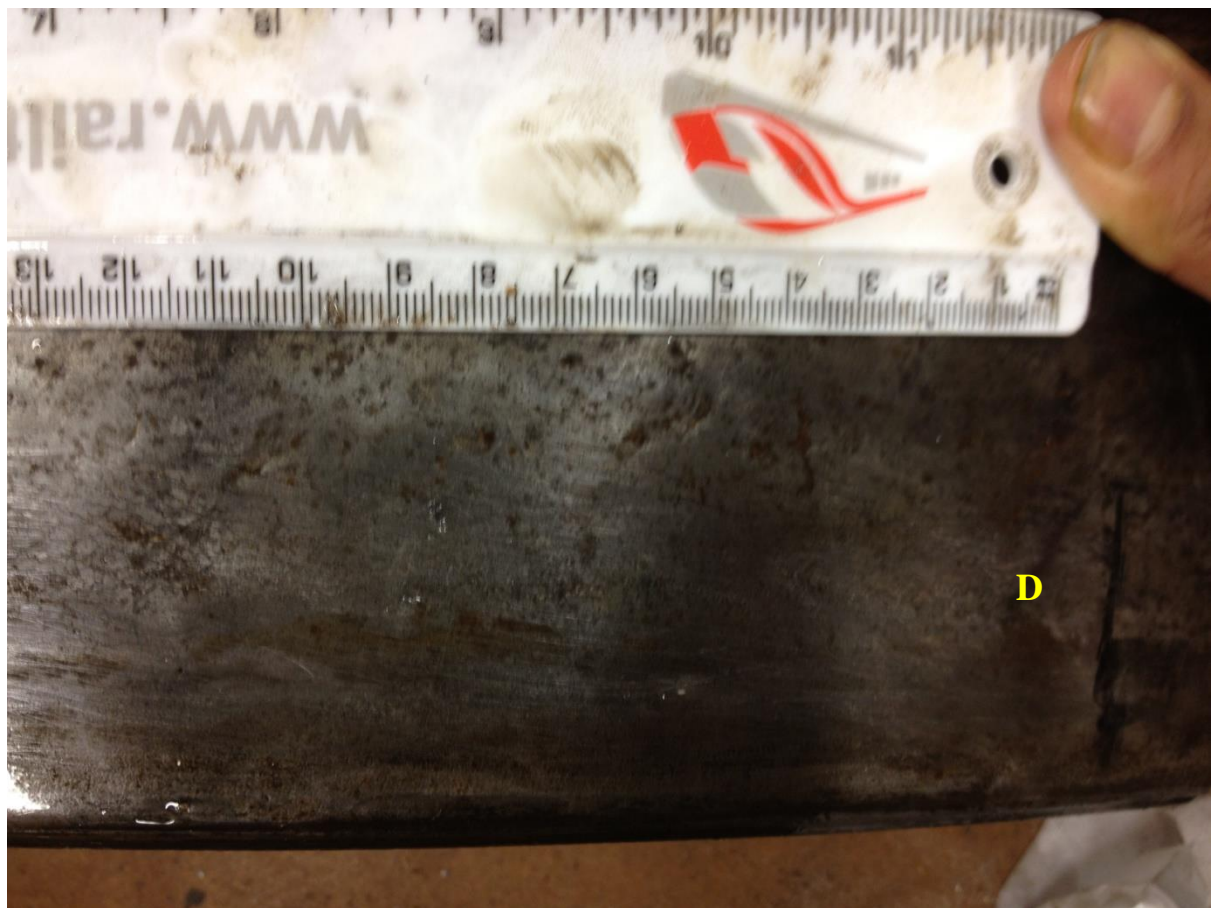
Figure 9.64 Feature D found on the tread of railway wheel HSR2 scanned by ACFM.
