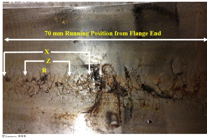
Figure 7.34 shows another image of the RCF prone region on the tread of wheel HSR1 showing the severe level of surface RCF damage that has occurred between 4 and 6 cm from the non-flange end of this wheel. Locations at which the subsequent ACFM scans (shown in the figures below) conducted on this wheel tread have been clearly labelled on the photograph.
