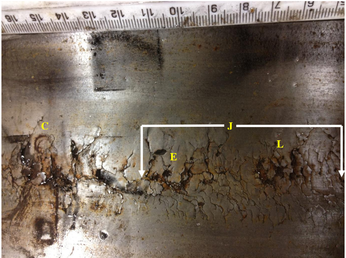
Figure 9.66 shows an image of the RCF prone region on the tread of wheel HSR1 showing the severe level of surface RCF damage that has occurred between 4 and 6 cm from the non-flange end of this wheel. Locations at which the subsequent ACFM scans (shown in the figures 9.65 and 9.66 below) conducted on this wheel tread have been clearly labelled on the photograph. Note that this figure is shown as figure 7.31 in chapter 7 of the PhD thesis above and has been reproduced here to keep it in context as it is part of this report and for the ease of the reader.
