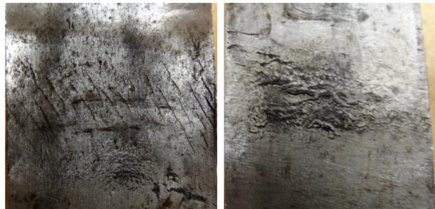
Figure 6.6 another high magnification photographs of the HSR2 railway wheel tread surface showing the two circumferential band of RCF cracks: first band consists of shallow and fine cracks oriented at approx. 60^{\circ} to the circumferential direction of the tread found near the flange and the second circumferential band of cracks are oriented almost perpendicular ( 90^{\circ} \pm 0.5^{\circ} ) to the circumferential direction of the tread and are found at approx. 3 cm from the non-flange end of the tread. These two bands of RCF cracks are regions of interest for the 3-D reconstruction of cracks using the multi-sectioning in conjunction with optical metallography approach and ACFM scans across these cracks as presented in chapters 4 and 6, respectively.
