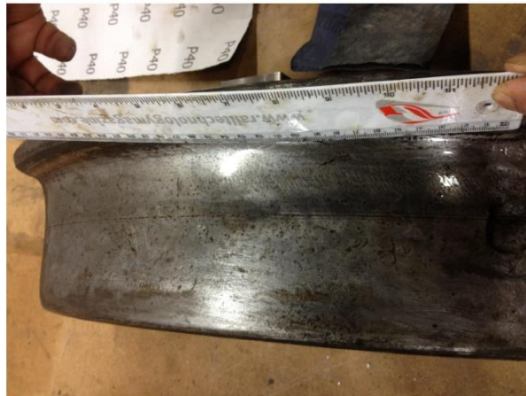
Figure 6.4 photograph of the HSR2 railway wheel tread surface showing the two circumferential bands of RCF cracks: first band consists of shallow and fine cracks oriented at approx. 60^{\circ} to the circumferential direction of the tread found near the flange and the second circumferential band of cracks are oriented almost perpendicular ( 90^{\circ} \pm 0.5^{\circ} ) to the circumferential direction of the tread and are found at approx. 3 cm from the non-flange end of the tread.
