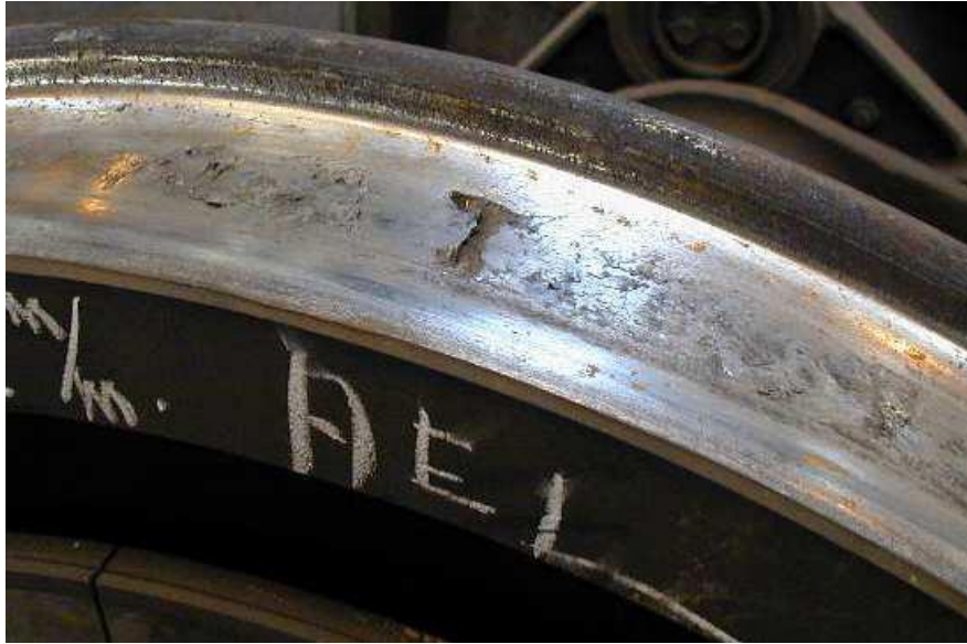
Figure 3.5(b): Figures 3.5(a) and (b) show a schematic and photograph, respectively, of local tread collapse in a railway wheel (the originals of the above schematic and photographic image are shown in reference [11] and have been reproduced and appropriately referenced here for the purpose of this PhD thesis).
