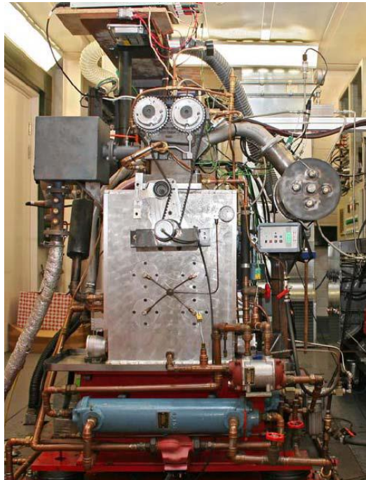
Figure 3-1 Thermal Single Cylinder Engine
