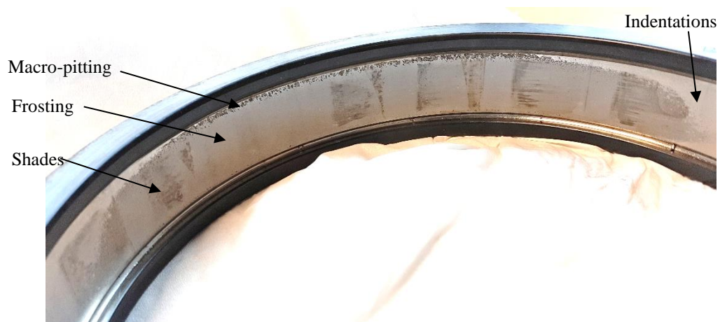
Figure 4.1.1-39 In the outer ring raceway, grey micro-pitted area (i.e. frosting), macro-pitting damage, separated light brown and dark grey shades, and small indentations were identified
