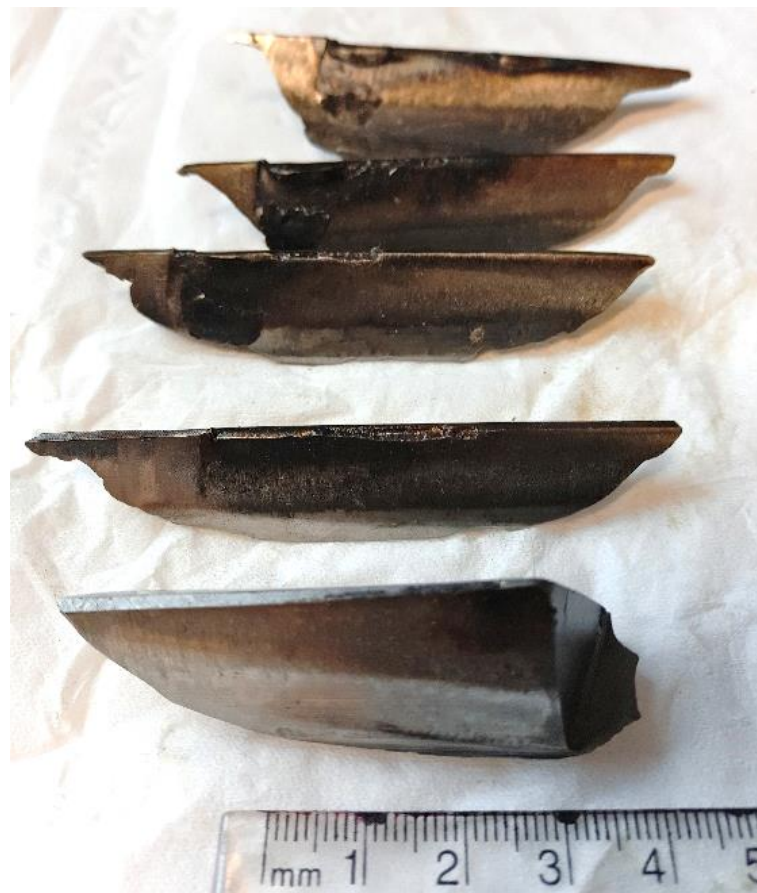
Figure 4.1.2-14 Five broken gear teeth from intermediate stage
