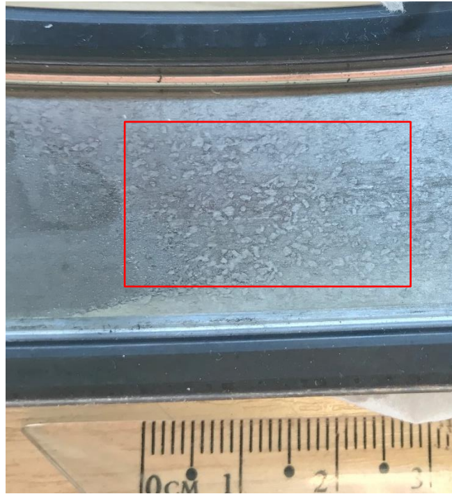
Figure 4.1.1-41 Closer observation of the small indentations by wear debris in the raceway, as framed
