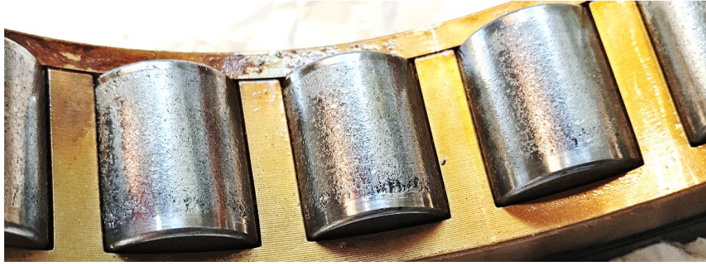
Figure 4.1.1-2 All the rollers are severely damaged
