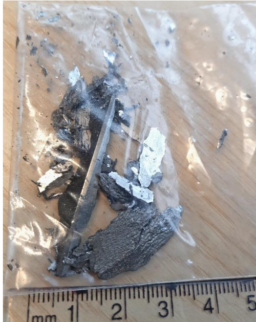
Figure 4.1.2-22 The debris from the low-speed planetary gears
