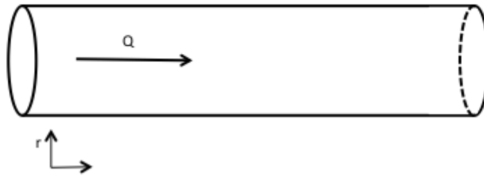
Figure 2.18: Simple schematic of a plug flow reactor
