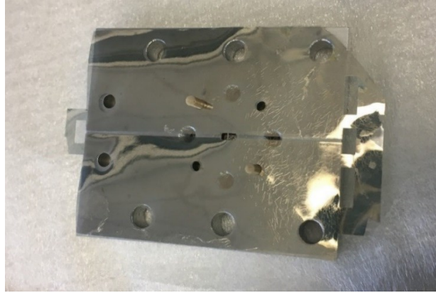
Figure 5.25: The thin film layer with 10nm silver deposited.
