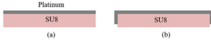
Figure 5.20: (a) surface deposition; (b) surface and side deposition of platinum on the SU-8 substrate
