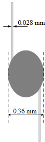
Figure 4.1: The bead thermistor from Sensor Scientific [3].
