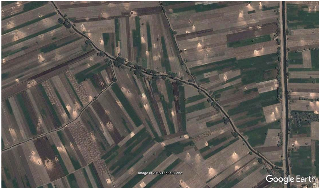
Figure 4.28: These field boundaries in 2011 between Manhari and El-Karm exemplify the arrangement of field boundaries perpendicular to local watercourses. The three drains flowing through the image provide irrigation water for the fields and so the channels flowing between each allotment must be able to receive the water from them.
