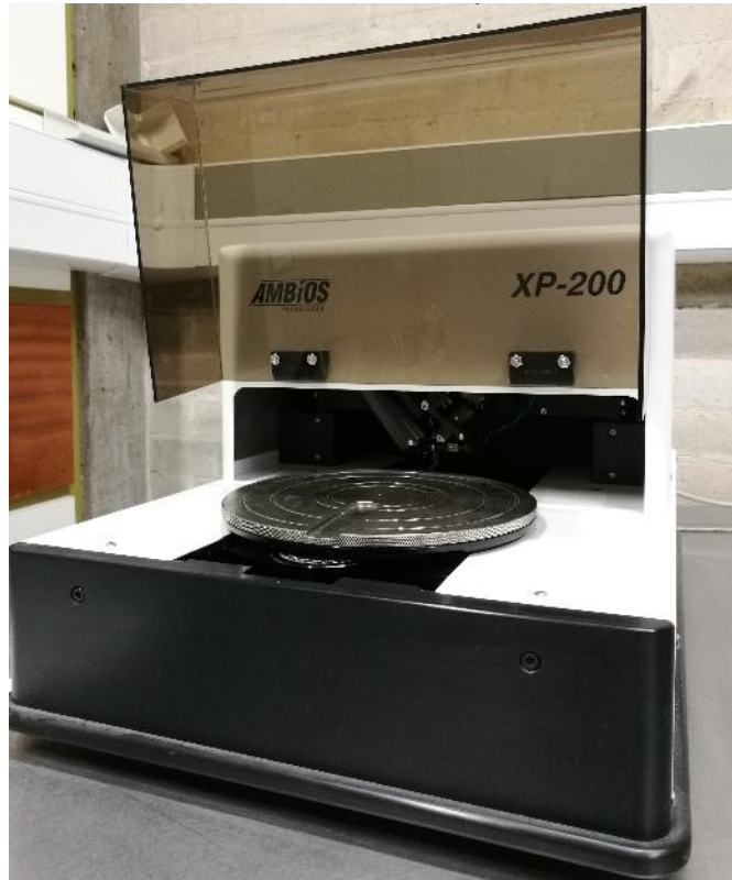
Figure 3.3 Digital photo of the 3D profilometer used for surface roughness measurements and wear track mapping.
