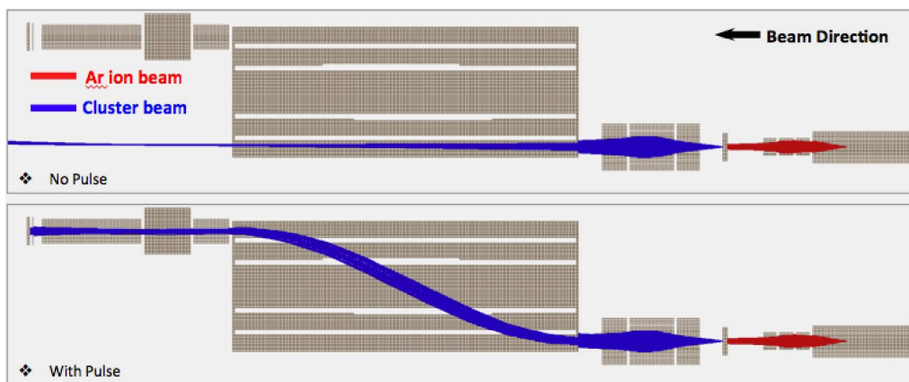
Figure 3.17: Schematic of the final ion optic setup for coupling the MACS source and the Von Issendorff-Palmer TOF mass-filter. The beam direction of travel is from right to left, the initial spread of the ions (red) is based on manual from the ISE-5 ion gun. The nanocluster initial trajectories are based on experimental data from the MACS1 running in transmission mode. The upper image shows direct focusing of the nanoclusters into the TOF spectrometer while all plates are grounded. The lower image is with the pulses switched on.
