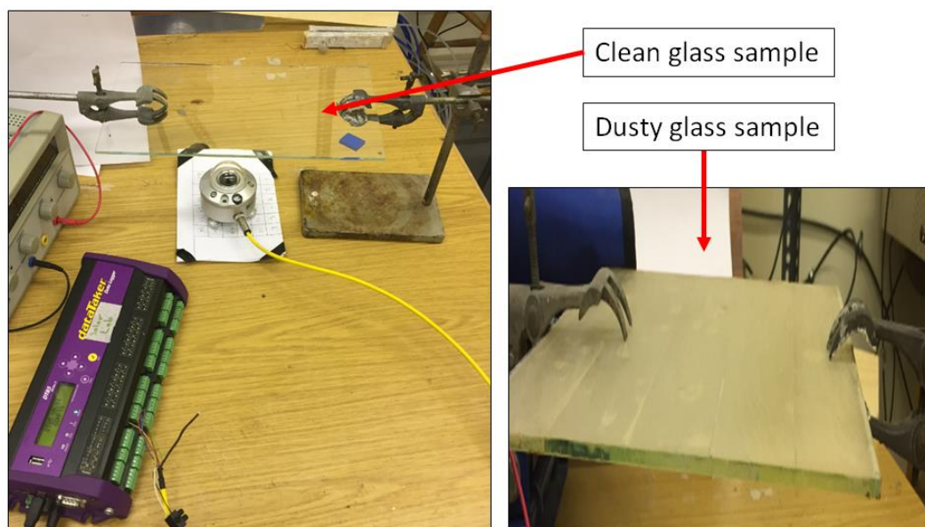
Figure 6.21 Photo of the measurement set up of the dusty glass transmittance
