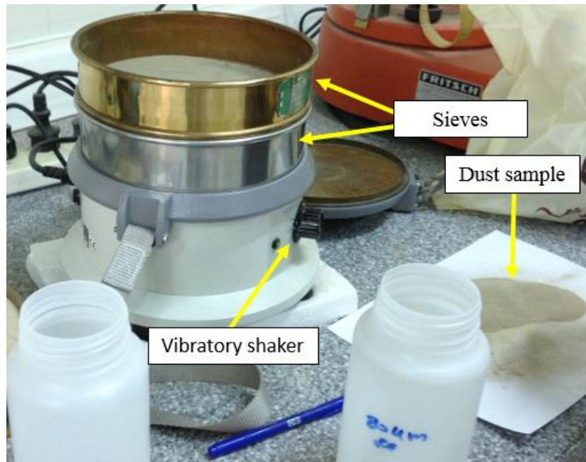
Figure 6.18 dust sample sieving test setup
