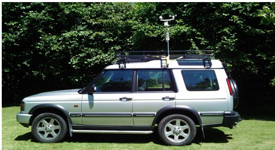
Figure 3.19: Portable weather station on the roof of Land Rover
