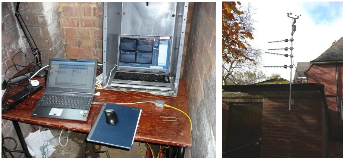
Figure 3.9: Central post (left – FSR data acquisition and video surveillance computers; right – receiving antennas for wireless cameras and weather station)
