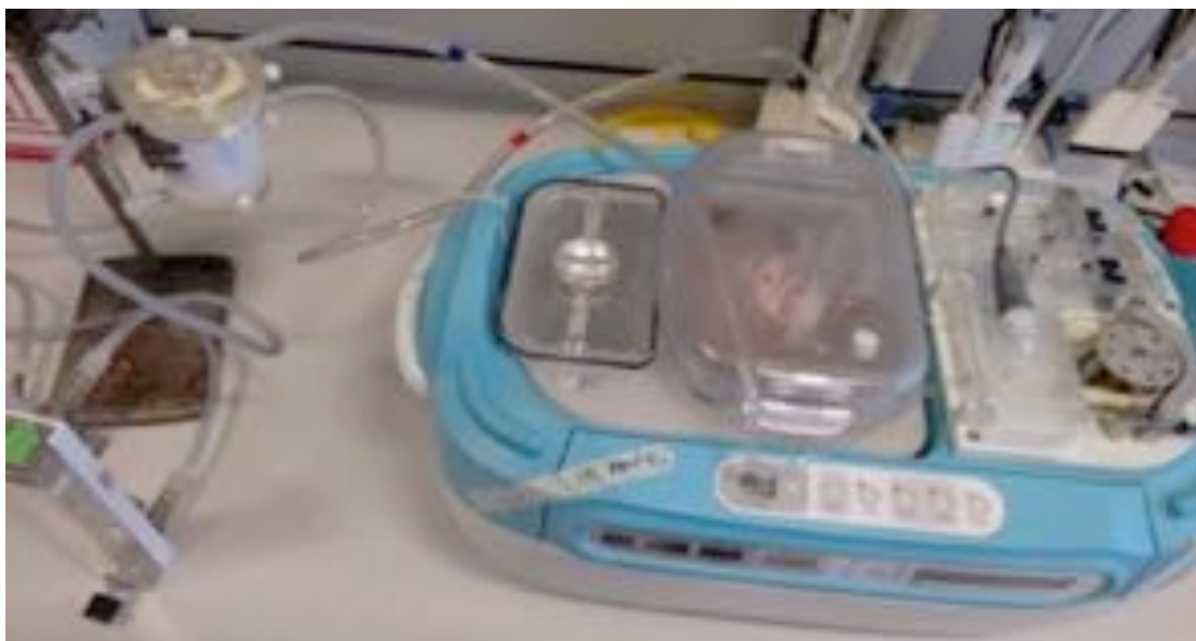
Figure 23 Modified LifePort© device with Hilite LT 800 paediatric oxygenator
