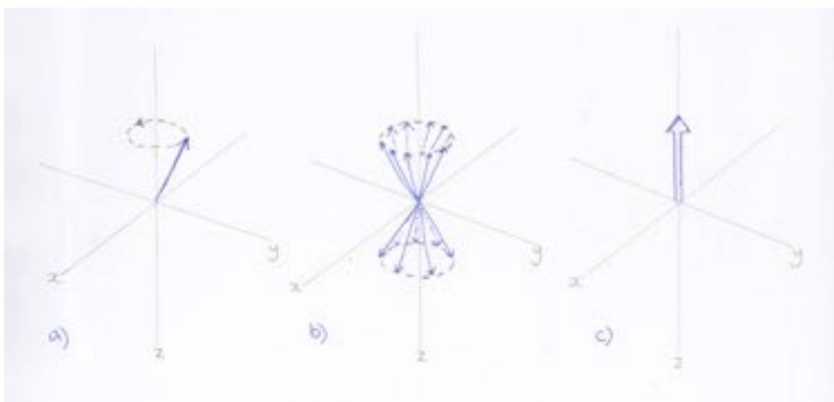
Figure 10 Mechanical vector model demonstrating the magnetisation vector of a single nucleus, multiple nuclei and the bulk magnetisation
