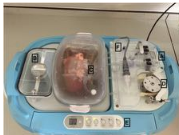
Fig. 1 LifePort Kidney Transporter 1.0 (Organ Recovery Systems) containing a porcine kidney. a Bubble chamber. b Reservoir for ice. c Aortic patch connector for perfusion. d Peristaltic pump. e Controls (pressure, prime, wash, infuse). f Sampling port
