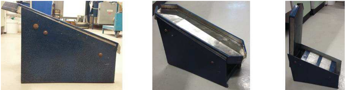
Figure 70. Wet low intensity magnetic separation system.
