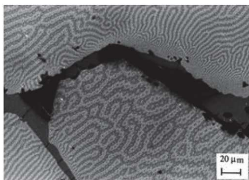
Figure 18. Kerr effect image of homogenised \text{Nd}_{16}\text{Fe}_{76}\text{B}_8 showing domain patterns. Reproduced from http://www.birmingham.ac.uk/Documents/college-eps/metallurgy/research/Magnetic-Materials-Background/Magnetic-Materials-Background-8-Domain-Observation.pdf Accessed 14/11/2016
