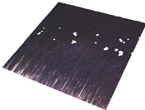
Figure 5.3-11 Surface morphology of an optimized sidewall produced in DRIE
