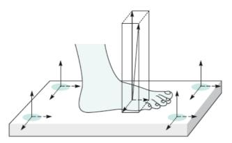
Figure 7. Kinetics gait analysis: Ground reaction forces of the foot strike on the instrumented force plate (Richards et al., 2013).
