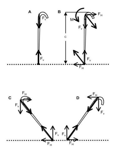
Figure 12. Illustration of the applied hand forces on the walking stick creating horizontal ground reaction force and therefore propulsion (B, C) and braking (D) in assisted locomotion. When the walking stick is in vertical position a moment (M) need to be exerted in order to create propulsion (A,B) and vice versa an opposite moment is required to brake. The walking stick users regulate propulsion and braking by holding the stick in different angles (C, D) (Bateni & Maki, 2005).
