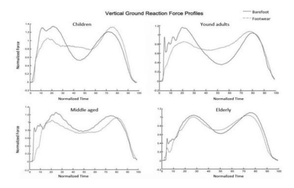
Figure 6. Vertical ground reaction force (normalized force to body weight) profiles illustrating the patterns of barefoot and shod walking in normalized time for the four age groups.
