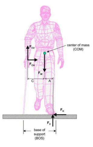
Fig 11. Illustration of walking stick use increasing the base of support during toe-off. (Bateni & Maki, 2005).
