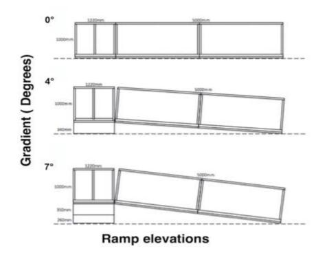
Figure 1. Custom-made wooden ramp elevations at 4 and 7 degrees.
