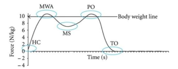
Figure 8. Profile of the shape of vertical ground reaction force during the stance phase of a normal gait pattern. Heel contact (HC), maximal weight acceptance (MWA), mid stance (MS), Push-off (PO), and Toe off (TO). (Bouffard et al., 2011)
