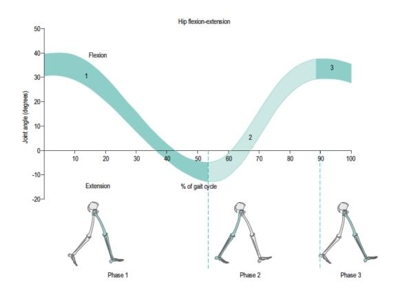
Figure 6. Hip flexion extension joint angle during the gait cycle (Richards et al., 2013)
