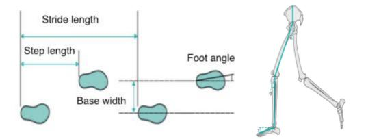
*Figure 3. Kinematics gait analysis: Definition of gait spatiotemporal parameters (left) and joint angle measurement (right)* (Richards et al., 2013)
