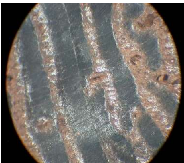
Figure 4x. Original size light microscopy image at a 40 x magnification of a Zebrano ( M ) untreated interior.
