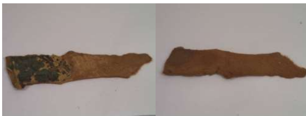
Figure 4.6. Two photographs showing the front (coated) and back of the untreated leather sample E.
