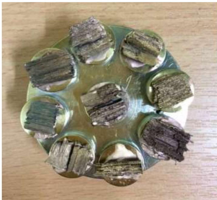
Figure 2.4. A photograph to show the wood samples mounted on the aluminium stubs using colloidal carbon cement.
