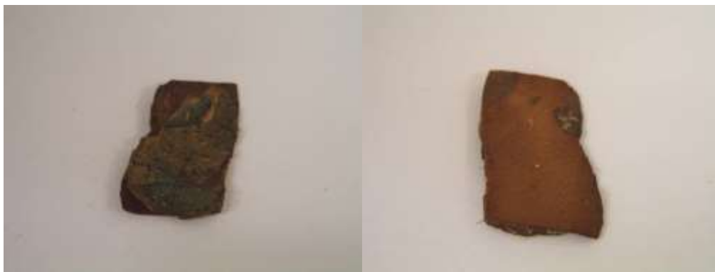
Figure 4.7. Two photographs showing the front (coated) and back of the treated leather samples F.
