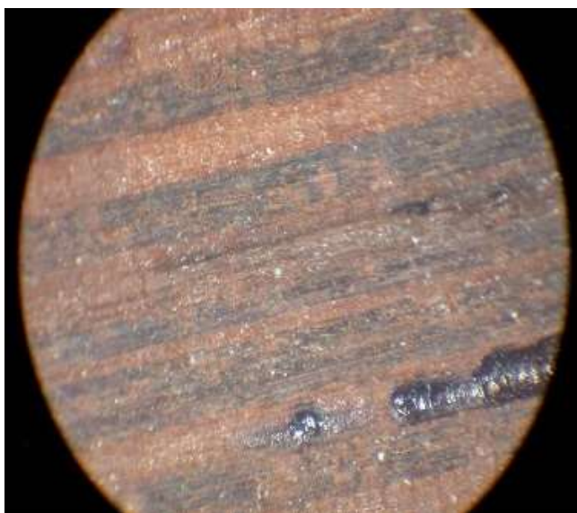
Figure 4w. Original size light microscopy image at a 40 x magnification of a Zebrano ( M ) untreated exterior.
