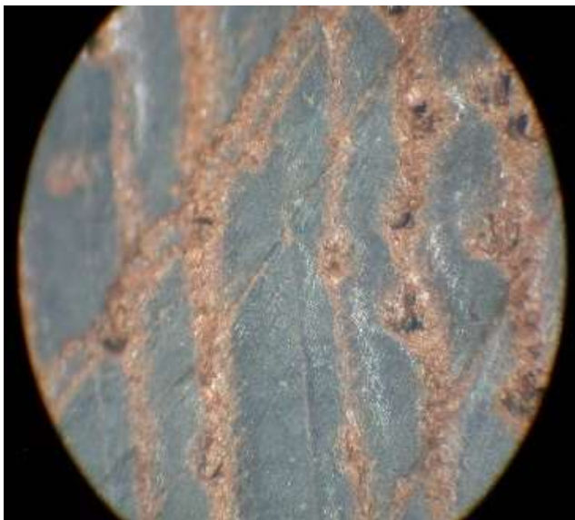
Figure 4ab. Original size light microscopy image at a 40 x magnification of a Zebrano ( M ) damaged interior.
