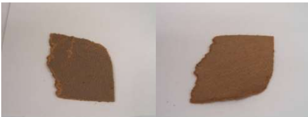
Figure 4.2. Two photographs showing the front (coated) and back of the untreated leather sample A.
