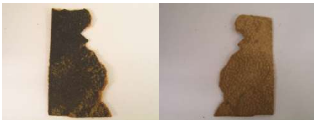
Figure 4.4. Two photographs showing the front (coated) and back of the untreated leather sample C.
