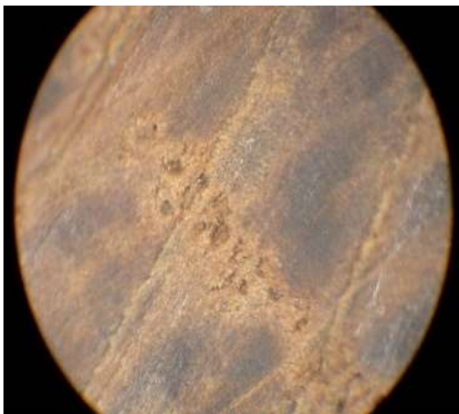
Figure 4d. Original size light microscopy image at a 40 x magnification of a White Oak ( H ) treated interior
