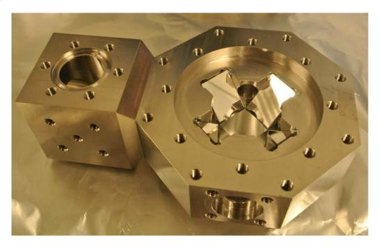
Figure 4.8: The octagonal chamber holds the prism mirrors for trapping the atoms. A valve, a dispenser and a ion pump with pumping speed of 2 L/s are connected to the vacuum setup through the cubic chamber. Some strontium oxide sample is held in the borehole which connects the octagonal chamber and the cubic chamber.
