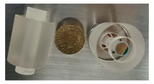
Figure 5.10: The cavities are multiband coated for stabilizing more than one laser in one cavity. The length of the ultra low expansion(ULE) cavity body is 30mm.
