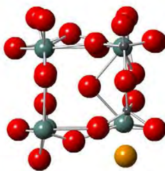
Figure 4.64: Oxygen Frenkel pair clusters associated with the site 1 position which include a polymerised phosphate unit. The vacancy site is highlighted in orange.
