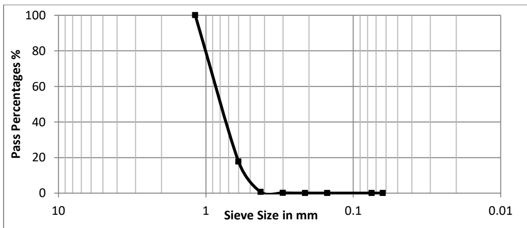
Figure 4.3: Sieve analysis of the Leighton Buzzard Sand used
