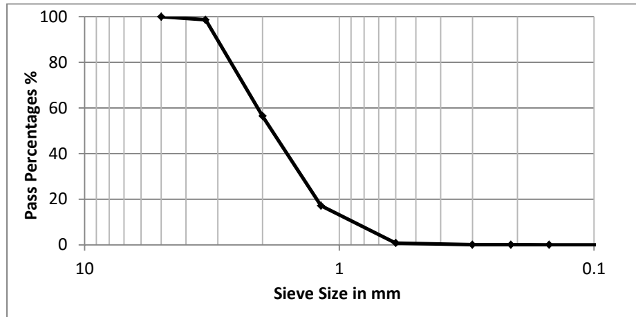
Figure 4.2: Sieve analysis for stone used as a fill material
