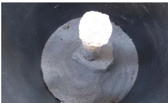
Figure 4.18: The cast column is ready to be studied for its failure shape after removing the surrounding soil
