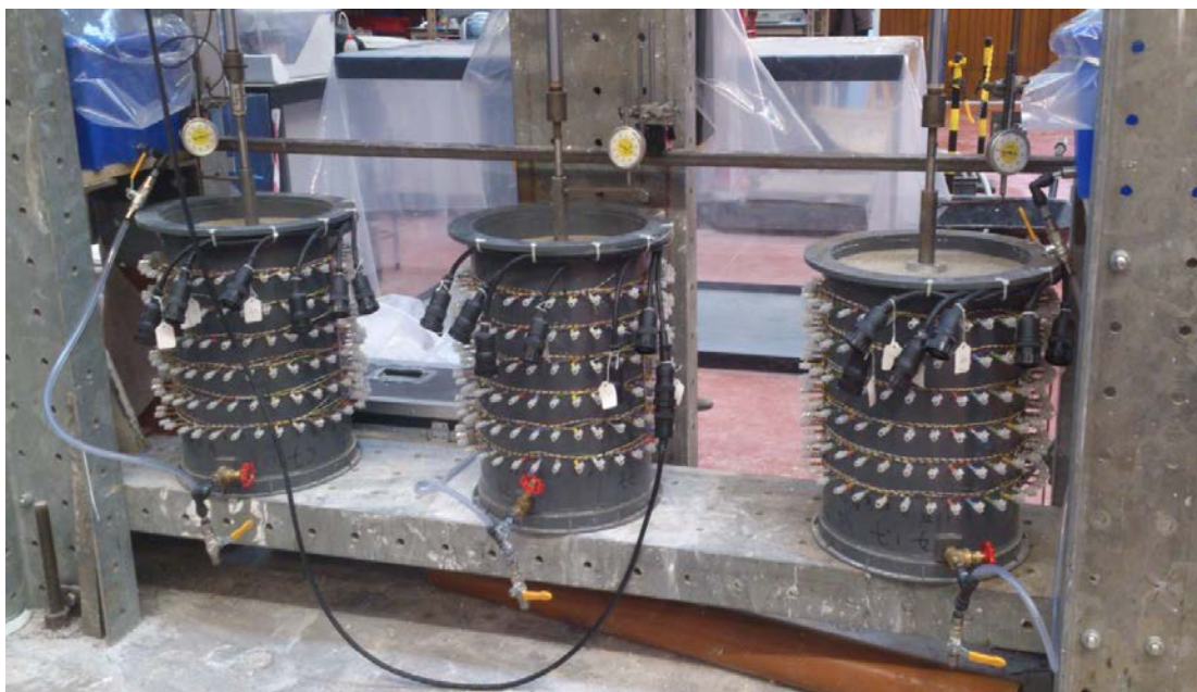
Figure 5.33: Providing the experiment with an inundation source and fixing the dial gauges in their positions
