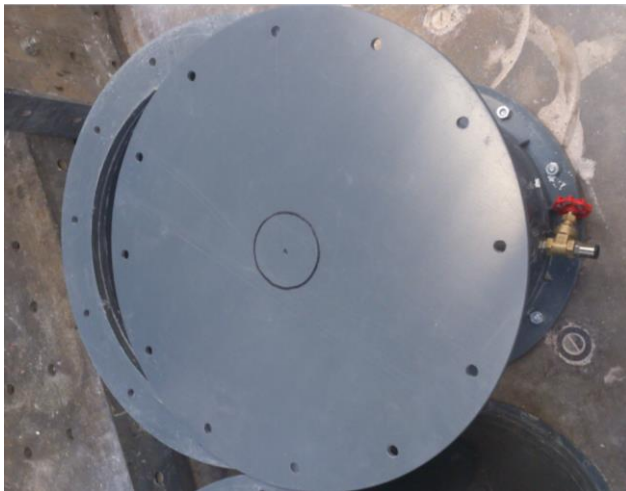
Figure 4.5: The PVC plate placed over the test cell used for load eccentricity
