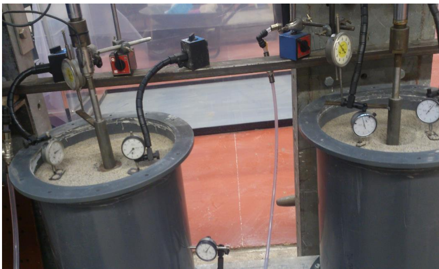
Figure 6.11: OSC (on right) and ESC (on left) under stress of 800 kPa
