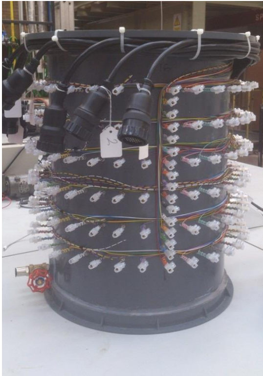
Figure 5.7: The resistivity cell after installing the wiring
