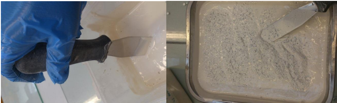
Figure 4.16: Left: Mixing the cast powder with water; Right: Mixing the cast paste with the vacuumed aggregate
