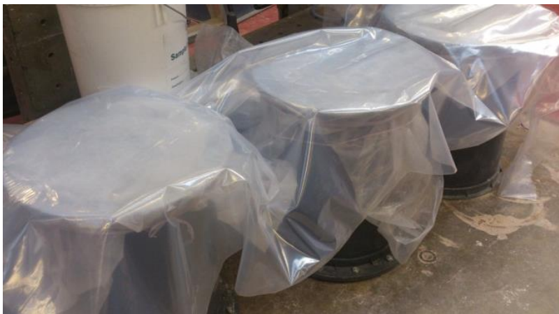
Figure 4.9: The three cells covered with three well-sealed nylon sheets after compacting
