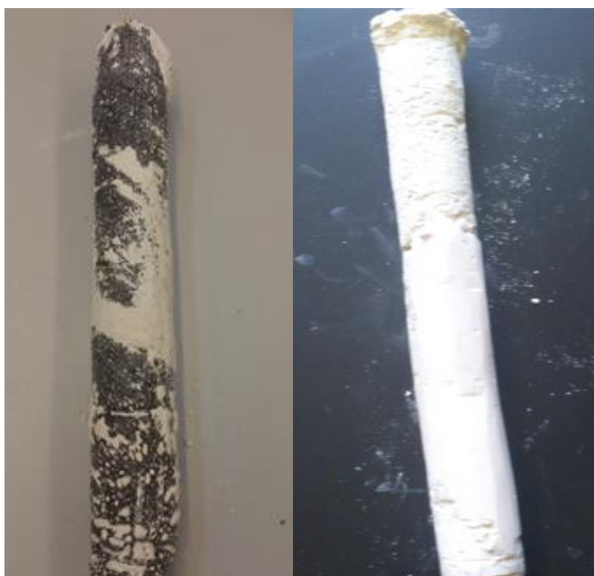
Figure 6.6: No bulging was observed for either OSC or ESC columns
