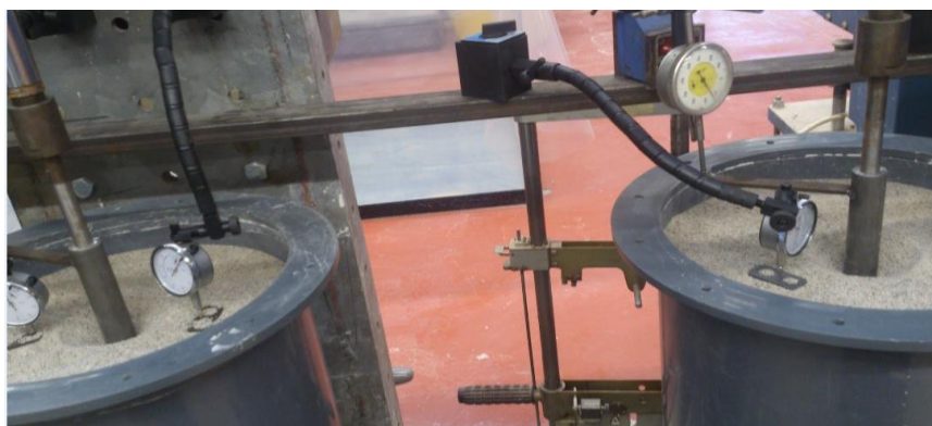
Figure 6.9: Untreated soil (on right) and OSC (on left) under stress of 800 kPa
