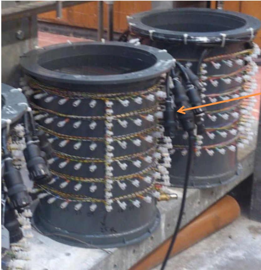
Figure 5.11: Measuring the resistivity of tap water using the acquisition system
