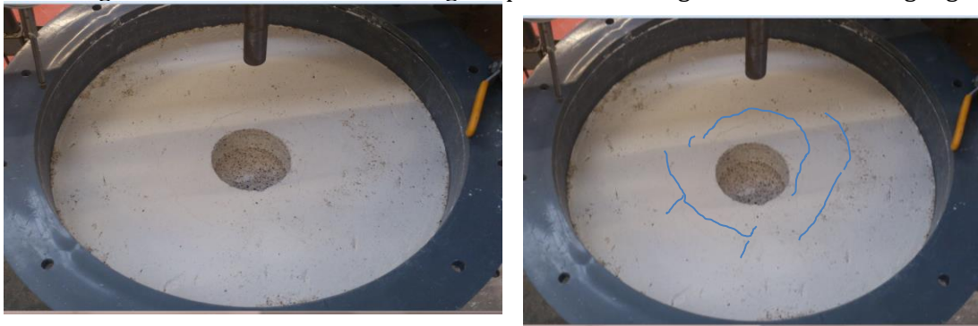
Figure 6.16: Cracks observed after completion of loading on untreated soil US and removing the foundation and sand layer, on left the original photo and on right the cracks are highlighted
