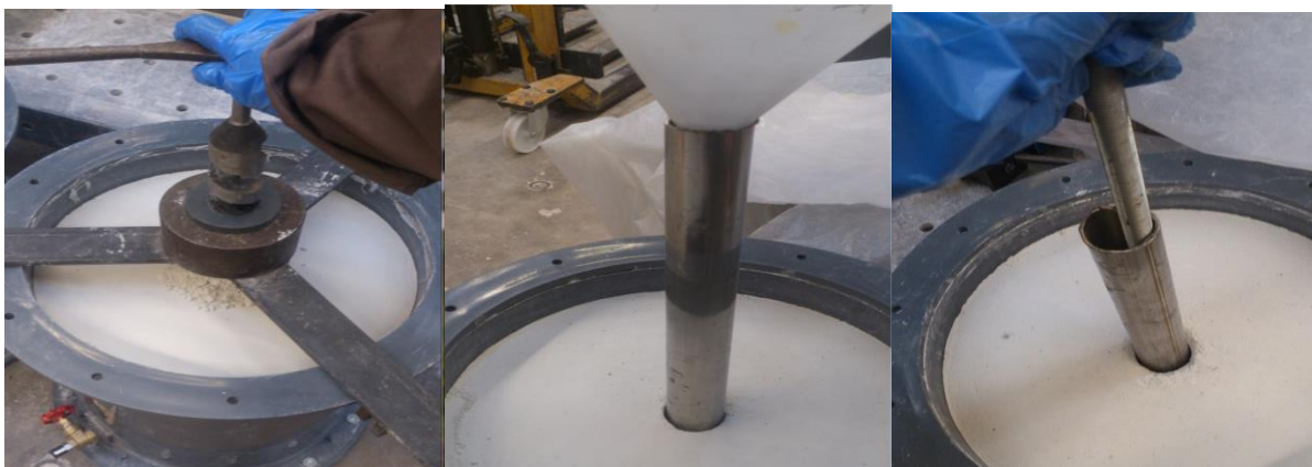
(a) The auger bit surrounded by the cross frame
