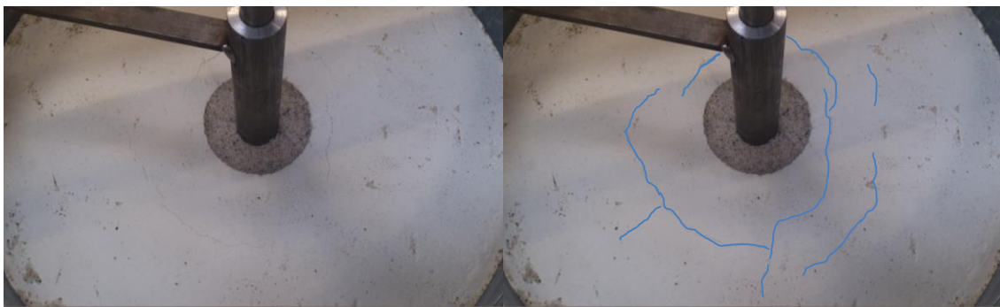
Figure 6.15: cracks observed after completion of loading on untreated soil US and before removing the foundation, on left the original photo and on right the cracks are highlighted
