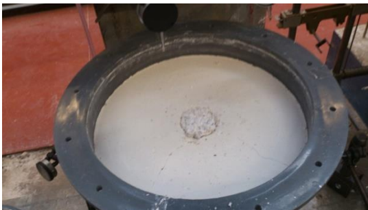
Figure 4.17: The cast paste was poured into the empty hole in the centre of the host ground
