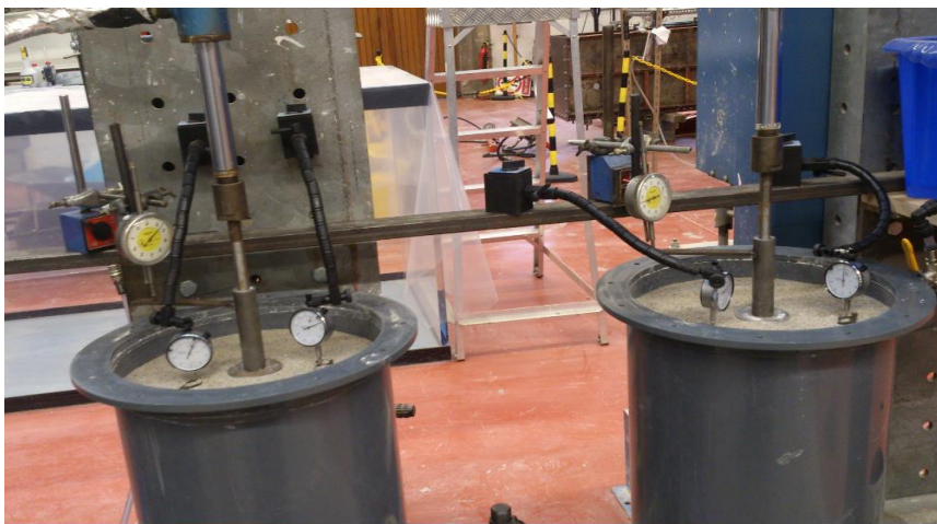
Figure 6.8 : Untreated soil (on right) and OSC (on left) under stress of 400kPa
