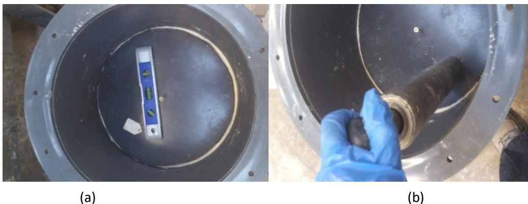
Figure 4.7 (a): The level of the plate is checked with a spirit level, (b): Compaction process using hammer
