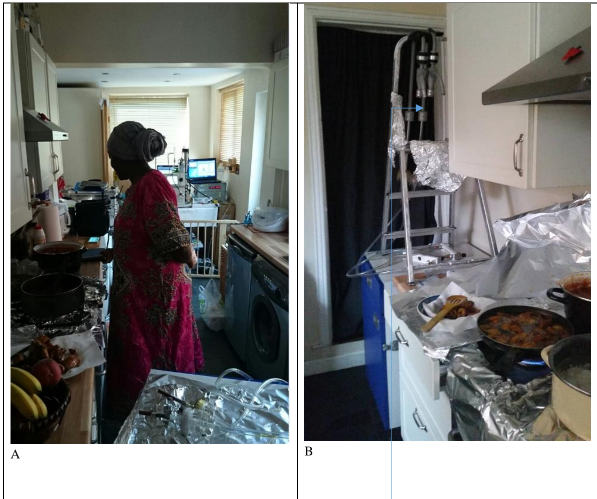
Figure 8 Sampling in home kitchen with extractor fan off ,A. without size selective inlet, B. with PM 2.5 inlet
