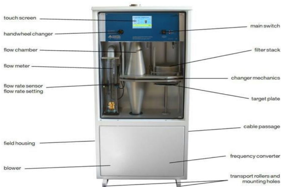
Figure 18 Hi-volume sampler unit of a Digital high-volume sampler (Enviro Technology Services Plc, n.d)
