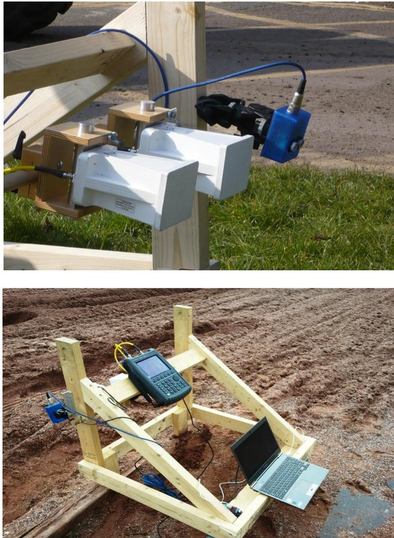
Figure 4.2: Radar and ultrasonic front-ends
