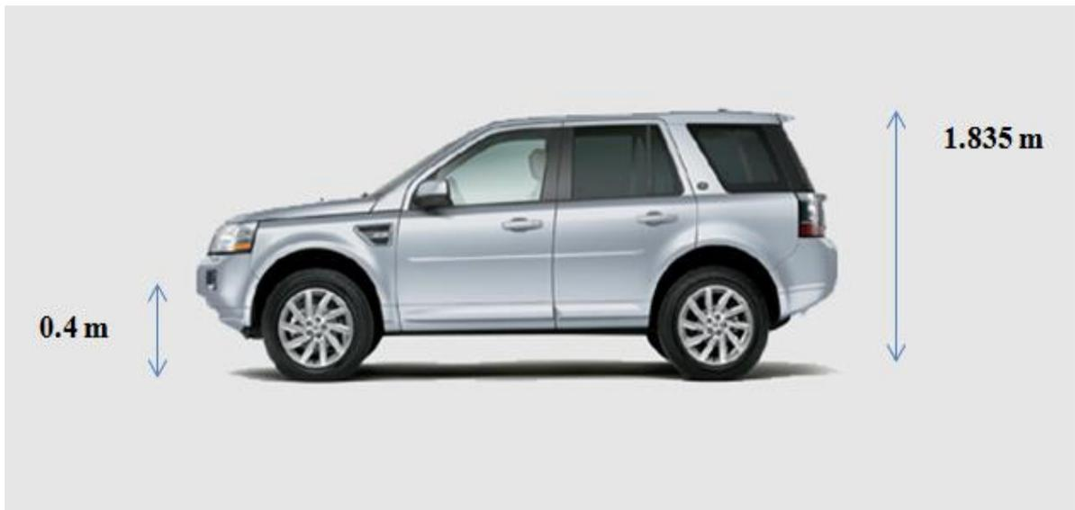
Figure 4.12: Range rover top and bumper height.
