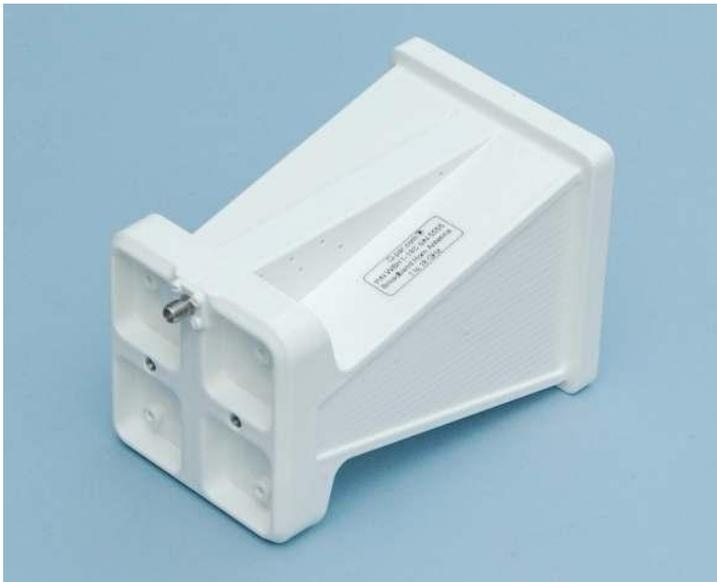
The photo above shows the back of the antenna, with weight reduction applied to the mounting plate. The photo also shows the two M5 mounting holes, spaced on 38 mm centres.
