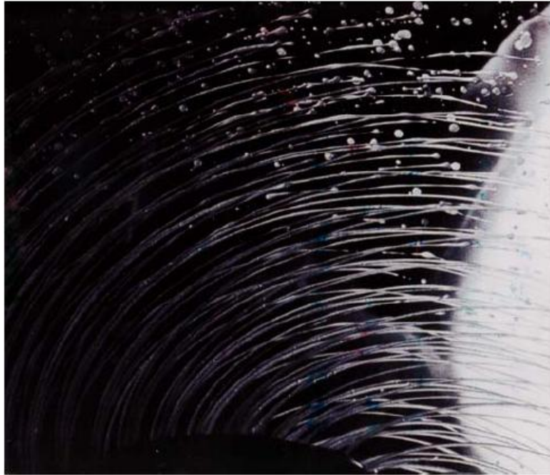
Figure 3.1: Photograph showing multiple jets emerging from a can (dark shape at the bottom of the photograph) in the prilling process. Some droplets can also be seen at the top of the photograph. Reproduced from Wallwork [45].
