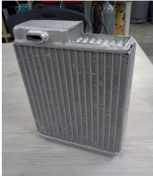
Figure 2.13 Finned rectangle TES device [127].
