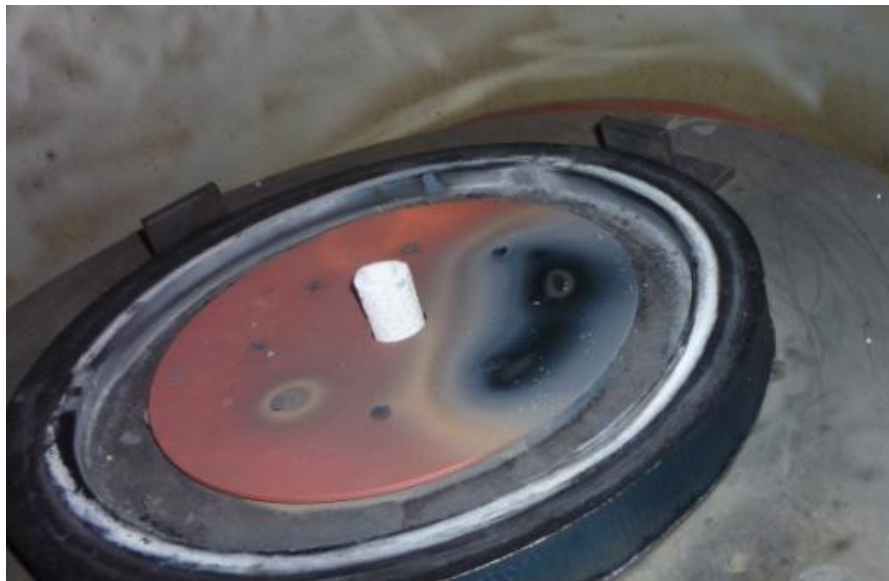
Fig 6.3. Deposits found on the copper baffle after withdrawal at 1300^{\circ}\text{C} .
