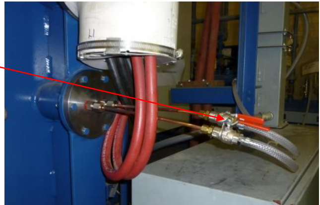
Fig. 5.6. Water pipes in and out of the Retech furnace providing water cooling for the copper baffle.
