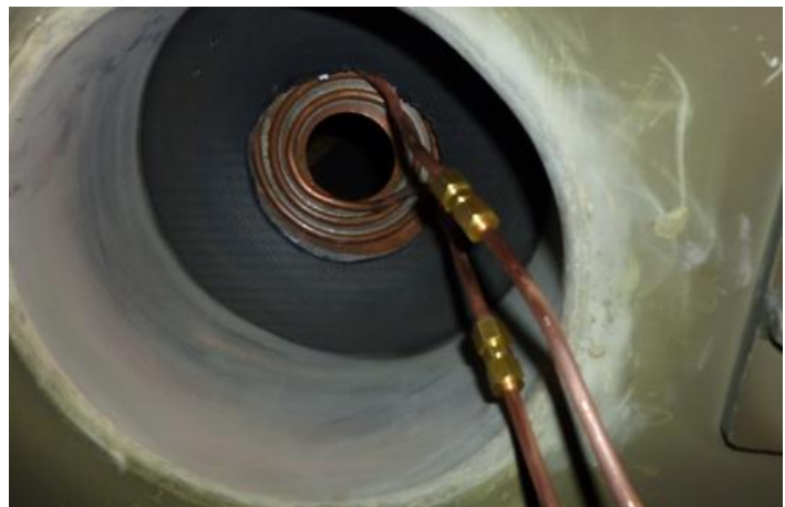
Fig. 5.8. Pipe connections made underneath the water cooled baffle. Note it was also possible to leave the insulation baffle in place.
