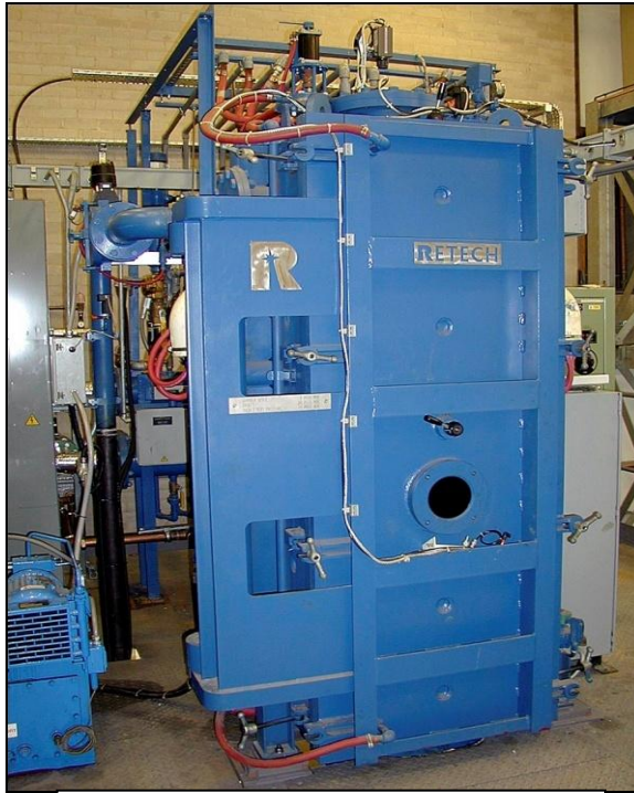
Fig. 1.2. The Retech single shot DS furnace at Birmingham University, donated by Rolls Royce plc.
