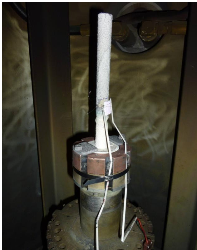
Fig. 5.4. Image showing the 20mm diameter cylindrical ceramic mould on the copper chill plate - thermocouples located in the mould to measure temperature.
