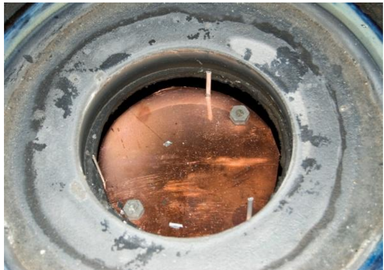
Fig. 5.2. Copper stand supporting three thermocouples under each baffle section.
