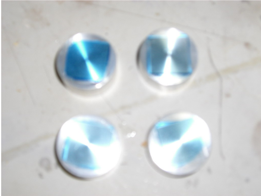
Figure 5.4 Glass slides bonded on the sample holder
