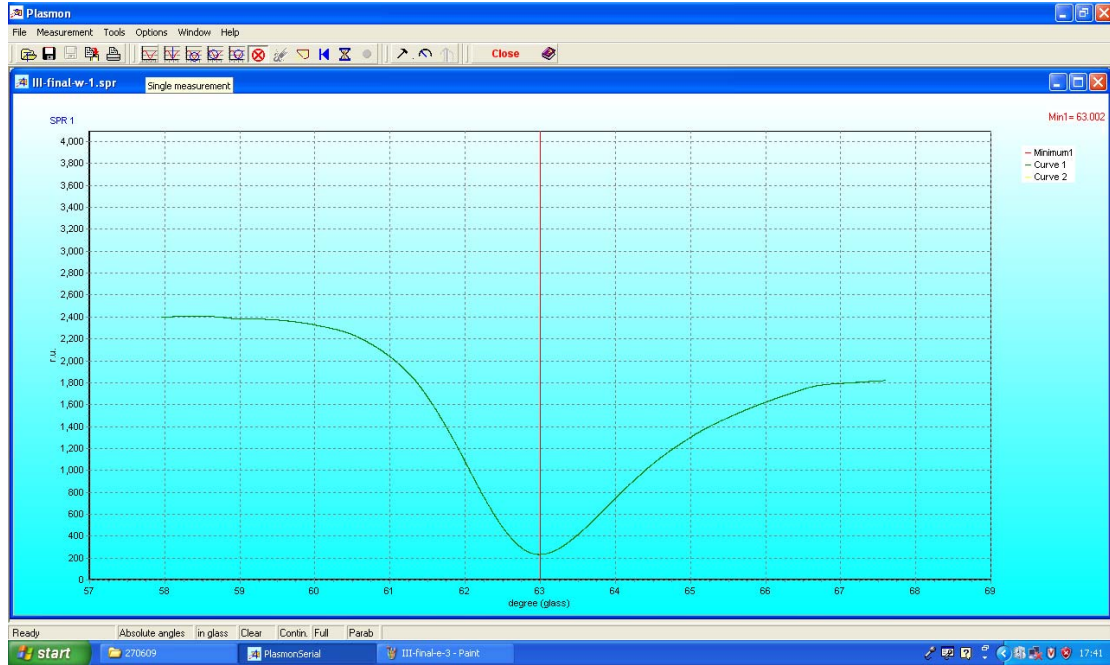
Figure C.1 SPR Curve 1 for glass 1, water as buffer solution
