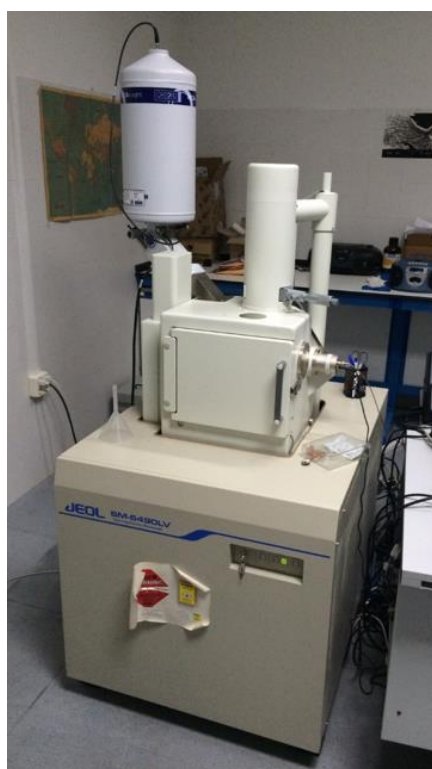
Figure 2-30 Scanning electron microscopy used for the measurements - JEOL SM-6490LV.
