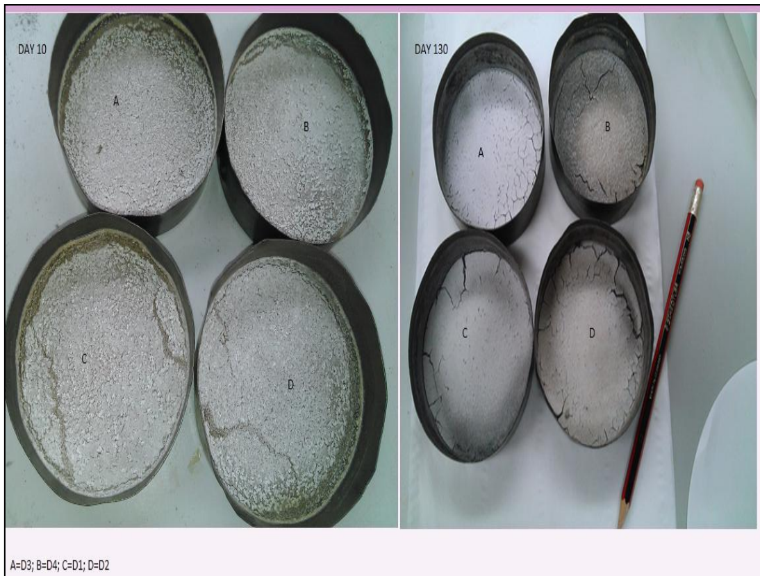
Figure B- 3. Change in total solids content of the sludge over time, A = D1, B = D2, C =D3 and D =D4.
