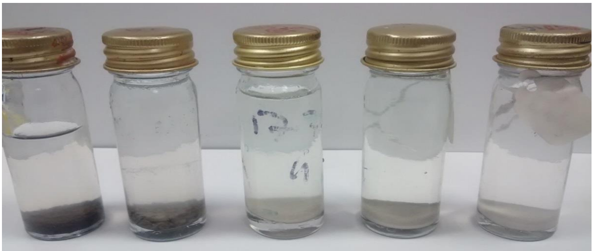
Figure 3.7. Effluent samples just after sampling from D1. L-R, day: 7, 22, 77,122, &158; (note absence of day 129)
