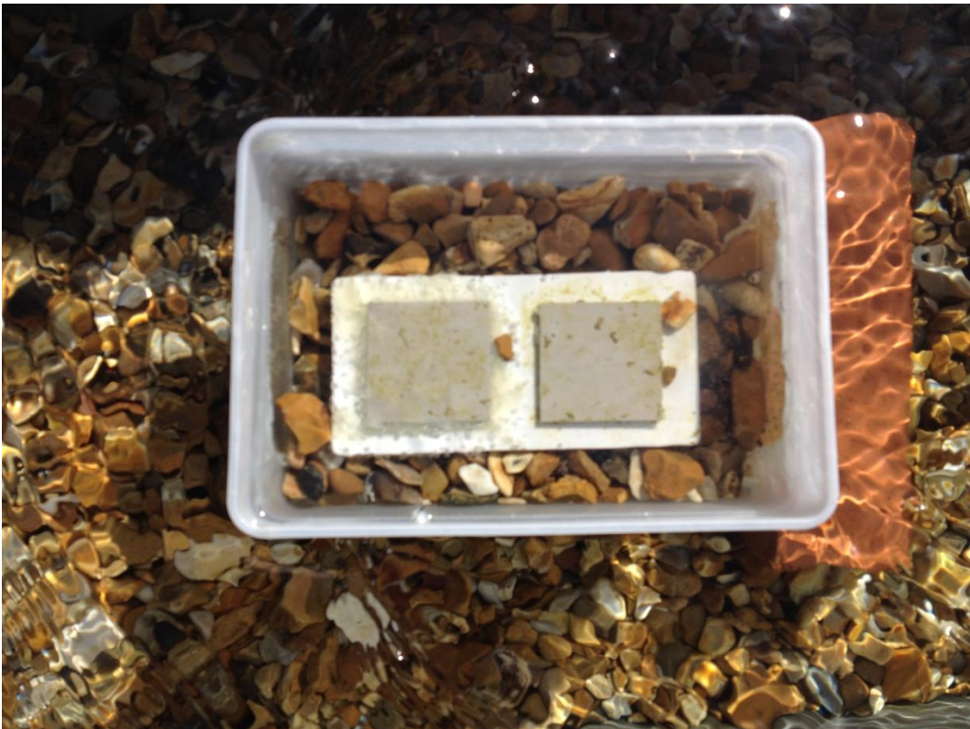
Figure 6.4. Microcosm with tiles and gravel inserted
