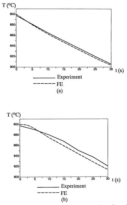
Fig. 7.5 Variation of billet temperature with time (transfer period) (a) near the surface (b) at the centre
