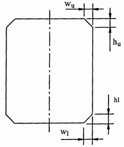
Fig. 5.2 Schematic illustration of a deformed billet in closed-die upsetting.
