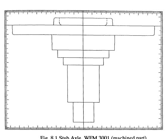
Fig. 8.1 Stub Axle, WFM 3001 (machined part)
