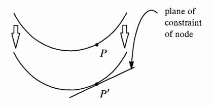
Fig. 4.5 Constraint of a node in contact with a translated die [52]
