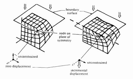
Fig. 4.6 Contact of a boundary surface with a node subject to previous constraining condition [52]
