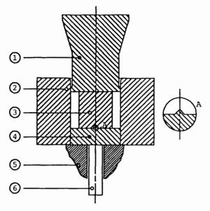
Fig. 5 Schematic illustration of the die-sets of closed-die upsetting (producing the 'cheese' from the 'billet'
