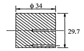
Fig. 7.6 Illustration of the billet used to obtain cooling curves (free resting period)
