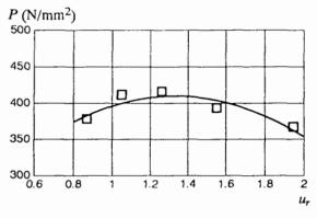
Fig. 6 Variation of average pressure with upset ratio for 2% unfilled die cavity (cheese diameter=41 mm) Fitted equation:
