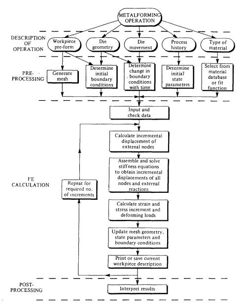
Fig. 4.1 Schematic illustration of the EPFEP3 analysis process [52]
