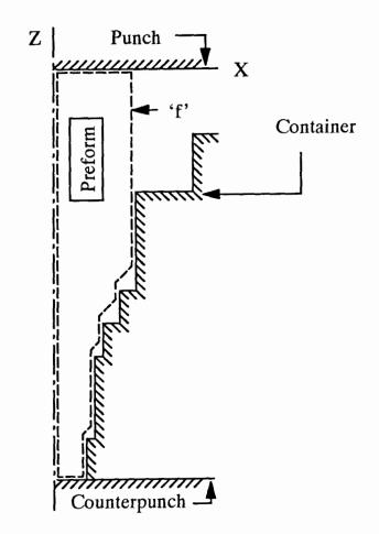
Fig. 4.15.a Schematic illustration of producing 'finish' from 'preform' (flat punch)
