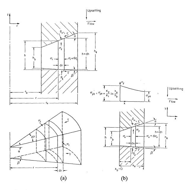
Fig. 2.6 Predicting stresses and load under inclined surfaces by using slab method [12]. (a) Axisymmetric (b) Plane strain
