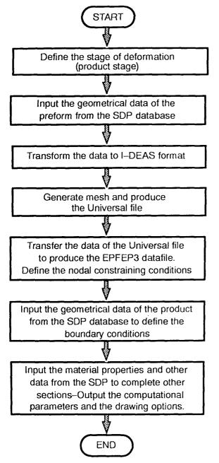
Fig. 3 The process of producing the EPFEP3 datafile.
