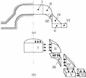
Fig 2.9 Schematic illustration of dividing half cross-section of an axisymmetric complex shape into simple shapes in UBET [40].
