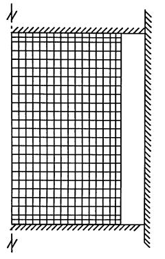
Fig. 7.1 FE mesh used to analyse the deformation (a half of the axial cross-section of billet, scale=2.5:1)
