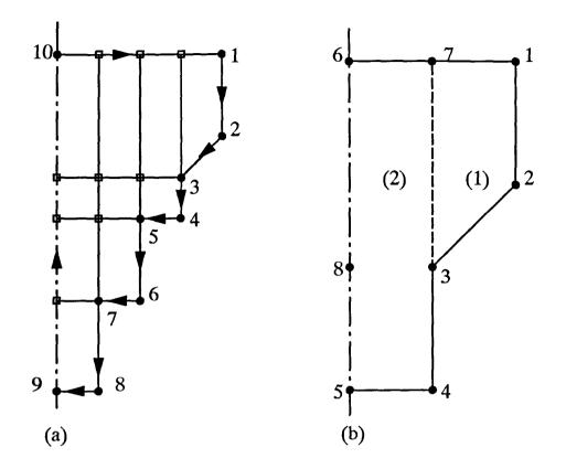
Fig. 4.11 Dividing the half cross-section of 'preform' to sub-areas to produce Mapped mesh
