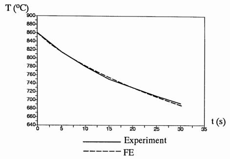
Fig. 7.8 Variation of billet temperature with time near the surface corresponding to Figs. 7.6 and 7.7
