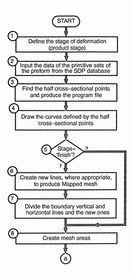
Fig. 4.8 The main actions of the mesh generation step
