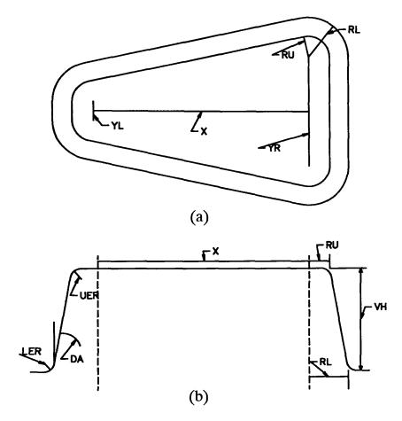
Fig. 3.1 The general definition of CONE (positive primitive) [92] (a) plan view (b) elevation
