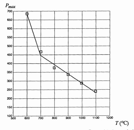
Fig. 5.14 Variation of maximum average pressure  $P_{max}$  with the workpiece<br/>pre-heat temperature T for forward extrusion- test No. 12.Fitted line:  $P_{max}(T)=823-0.536 T$  $700 < T < 1100 \ ^{\circ}C$ Fitted line:  $P_{max}(T)=2106-2.37 T$  $600 < T < 700 \ ^{\circ}C$
