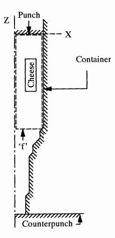
Fig. 4.14 Schematic illustration of producing 'preform' from 'cheese'
