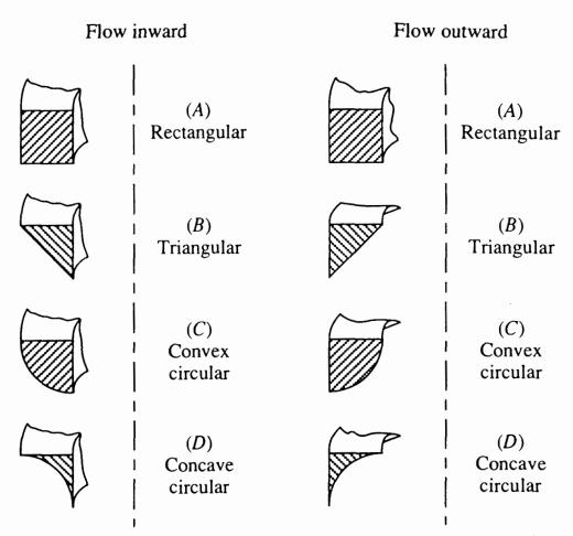
Fig. 2.8 Eight basic elemental rings in the analysis by UBET [40].
