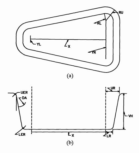
Fig. 3.3 The general definition of PLUG (negative primitive) [92] (a) plan view (b) elevation
