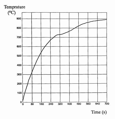
Fig. A.2 Heating curve for the centre of the billet Temperature of furnace: 900 °C
