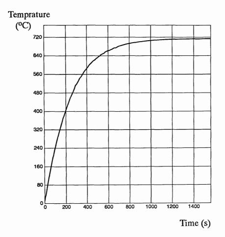
Fig. A.4 Heating curve for the centre of the first example Temperature of furnace: 720 °C
