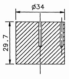
Fig. A.1 Billet used for experimental calibration curves (Example No. 1 in table 5.1)
