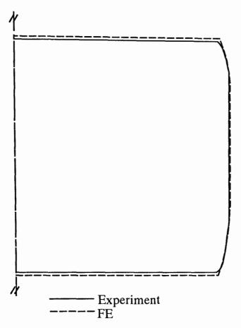
Fig. 7.11 Comparison between the geometry of the workpiece and that of the mesh, in the stage of corner filling (scale=4:1)
