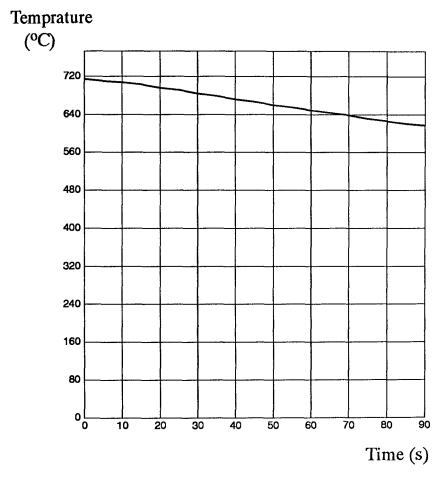
Fig. A.6 Cooling curve for near the surface of the billet Temperature of furnace: 720 °C
