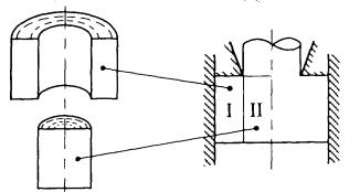
Fig. 2.7 Dividing an extrusion forging into a ring and a cylinder based on the UBET [39]
