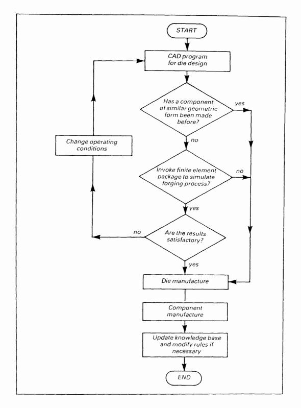
Fig. 2.14 A brief illustration of a forging Expert System [86], [87] and [88].
