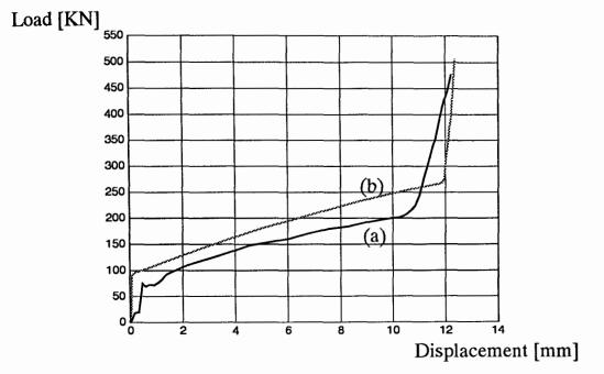
Fig. 8.8 Load-displacement curves obtained from experiment and simulation corresponding to Fig. 8.7.(a) Experiment (b) FE
