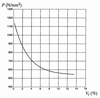
Fig. 5.5 Variation of average pressure P with unfilled corner volume  $V_c$ (test No. 1) –Fitted equation:  $P(V_c)=539+645.5e^{-0.326Vc}$
