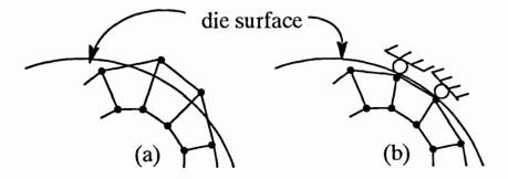
Fig. 4.4 Checking for contact between FE mesh and boundary surface (a) at the end of increment, (b) after checking for contact with die [52]
