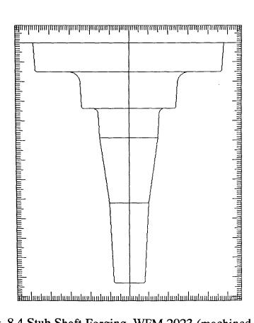
Fig. 8.4 Stub Shaft Forging, WFM 2023 (machined part)
