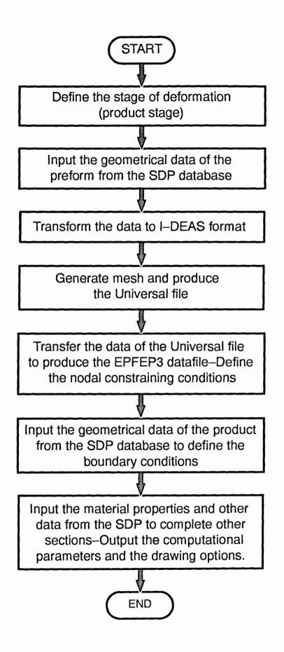
Fig. 4.7 The process of producing the EPFEP3 datafile
