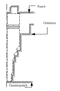
Fig. 4 Schematic illustration of producing the 'finished' part from the 'preform'.
