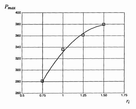
Fig. 5.13 Variation of maximum average pressure  $P_{max}$  with initial height/diameter ratio  $r_i$  for forward extrusion- test No. 9. Fitted curve:  $P_{max}(r_i)=19+459 r_i-146r_i^2$
