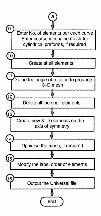
Fig. 4.8 The main actions of the mesh generation step (continued)
