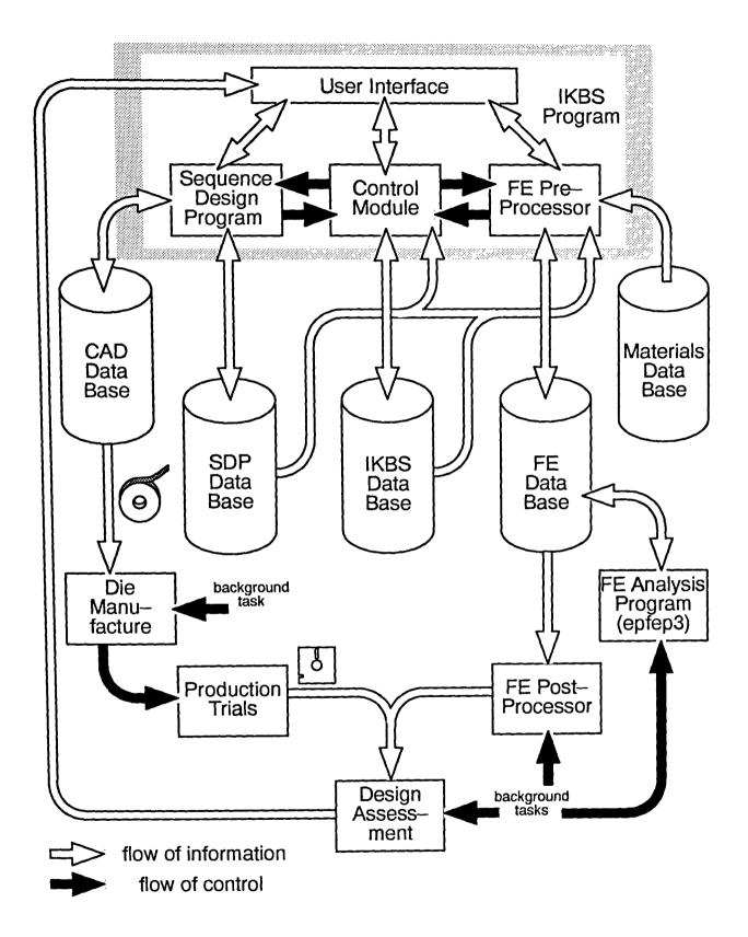
Fig. 2.15 The structure of an IKBS for the design of forging dies [91].
