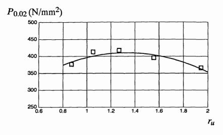
Fig. 5.6 Variation of average pressure at 2% unfilled die cavity ( $P_{0.02}$ ) with upset ratio  $r_u$  for closed-die upsetting-test No. 2 Fitted equation:  $P_{0.02}(r_u)=185.8+338.2 r_u-126.9 r_u^2$
