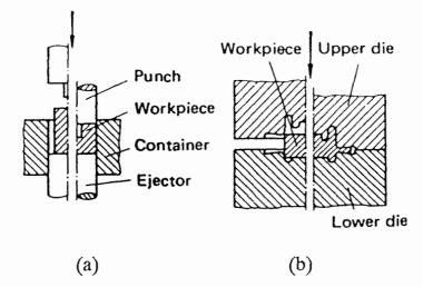
Fig. 2.1 Types of closed-die forging [6].(a) Completely closed-die (without flash)(b) Closed-die with flash (conventional)
