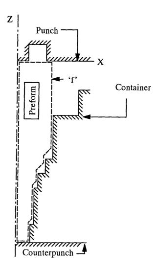
Fig. 4.15.b Schematic illustration of producing 'finish' from 'preform' (upper and lower dies)
