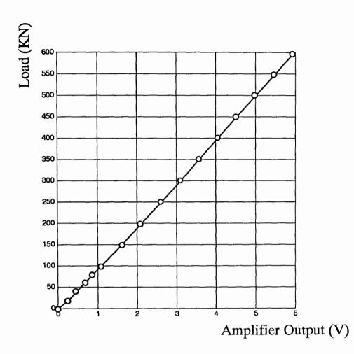
Fig. A.10 Load-cell calibration curve
