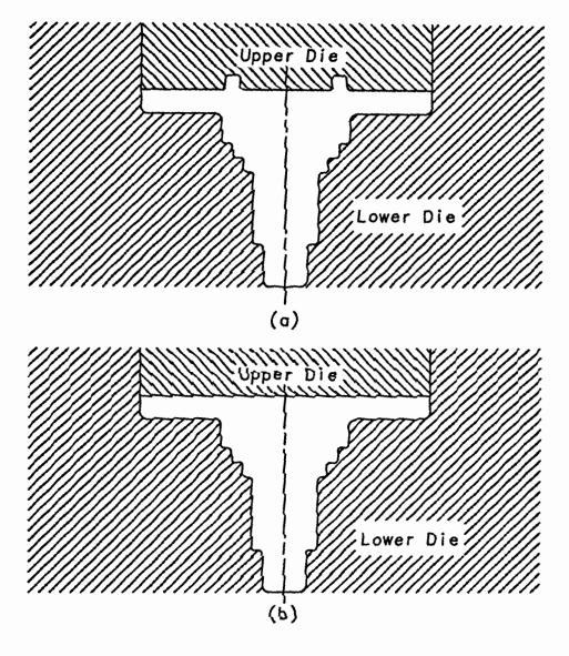
Fig. 3.6 Die types for finishing of two Stub Axle types [92] (a) Punch shaped to suit Stub Axle features
