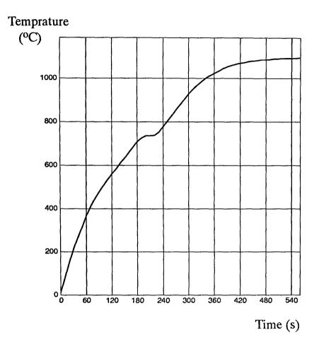
Fig. A.5 Heating curve for the centre of the billet Temperature of furnace: 1100 °C
