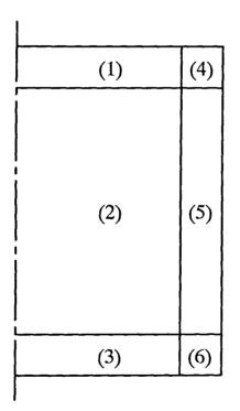
Fig. 4.10 Dividing the half cross-section of a cylindrical preform to 6 mesh areas when a fine mesh is required
