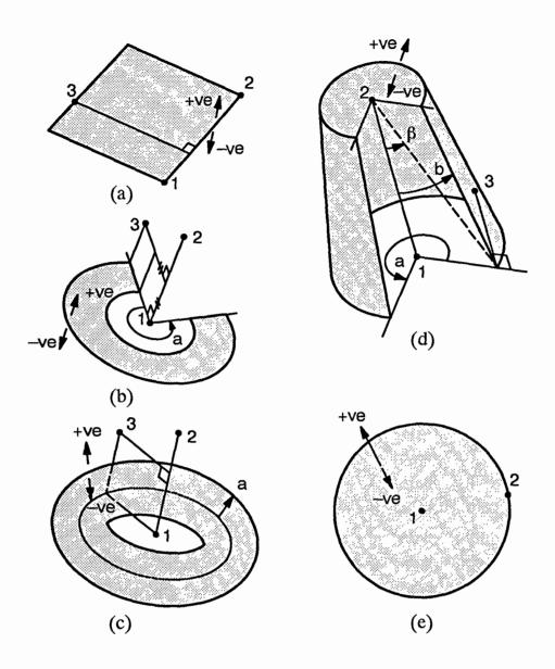
Fig. 4.3 Primitive geometric surfaces used in EPFEP3 [45] (a) rectangle (b) annulus (c) torus (d) cone (e) sphere
