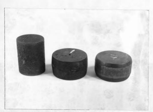
Fig. C.1 The geometry of the specimens in closed-die upsetting Left to right: billet (test piece no. 3 of test no. 2), the deformed workpiece just after making contact with the die wall, and the deformed workpiece at the stage of corner filling.
