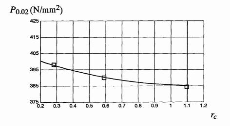
Fig. 5.7 Variation of average pressure at 2% unfilled die cavity ( $P_{0.02}$ ) with cheese ratio (height/diameter of the product  $r_c$ ) for closed-die upsetting- test No. 3 Fitted equation:  $P_{0.02}(r_c)=407.7-39.5 r_c+17.6 r_c^2$
