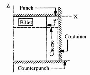
Fig. 4.13 Schematic illustration of producing 'cheese' from 'billet'
