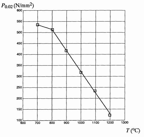
Fig. 5.9 Variation of average pressure at 2% unfilled die cavity ( $P_{0.02}$ ) with billet pre-heat temperature T for closed-die upsetting- test No. 5.
