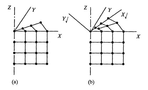
Fig. 4.9 Generating 3–D mesh for Stub Axles (a) unacceptable (b) acceptable
