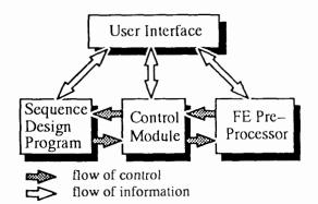
Fig. 1 The main parts of the IKBS for Forging Die Design [10].
