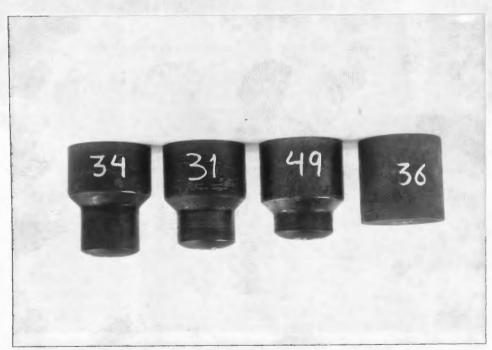
Fig. C.2 The geometry of the specimens in forward extrusion Right to Left: billet (test no. 8), and the deformed workpieces with different ratios of height/diameter of the extrudate.
