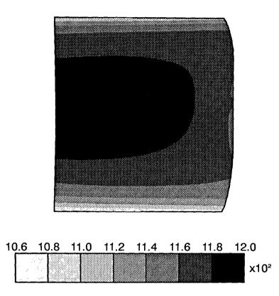
Fig. D.6 Absolute temperature (K) contours corresponding to Fig. 7.12.
