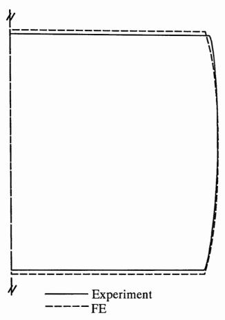
Fig. 7.9 Comparison between the geometry of the workpiece and that of the mesh, just when contact with the die is being made (scale=4:1)
