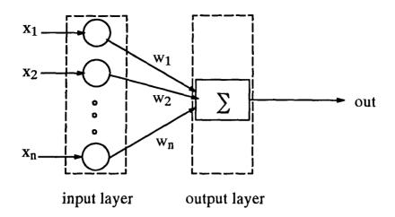
Fig. 2.12 A two layer single neuron Neural Network [84]
