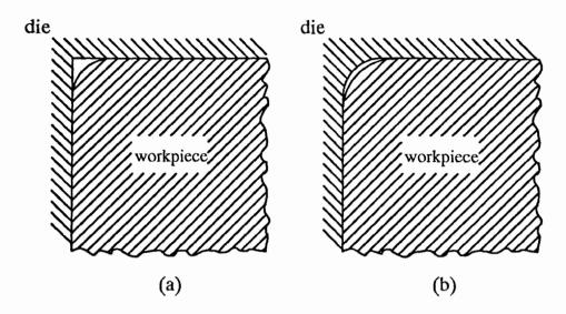
Fig. 5.4 Illustration of workpiece corner geometry in two different dies
