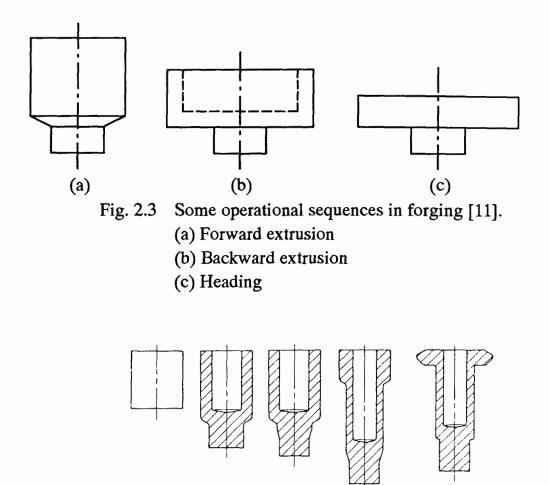
Fig. 2.4 Schematic illustration of operational sequences for a gear blank [4]. Left to right: billet, simultaneous forward and backward extrusion, forward extrusion, backward extrusion, simultaneous upsetting of flange and coining of shoulder.
