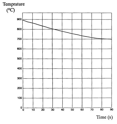
Fig. A. 3 Cooling curve for near the surface of the billet Temperature of furnace: 900 °C
