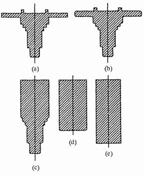
Fig. 2 The operational sequences for a Stub Axle
