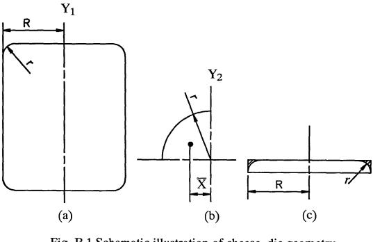
Fig. B.1 Schematic illustration of cheese-die geometry
