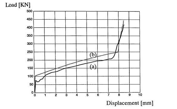
Fig. 7.13 Load-displacement curve obtained from experiment and simulation (a) Experiment (b) FE
