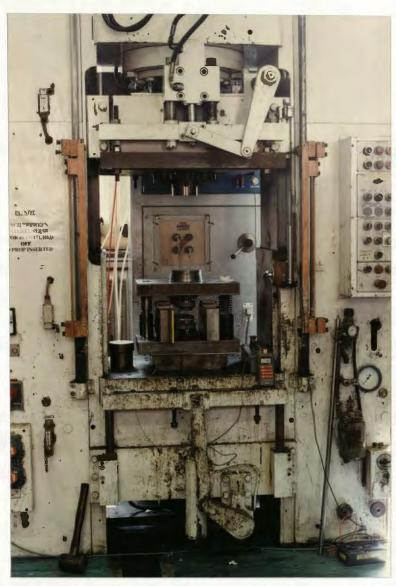
Fig. C.5 The 1500 KN hydraulic press used in the experiments.
