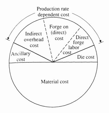
Fig. 2.2 The distribution of forging cost [7]
