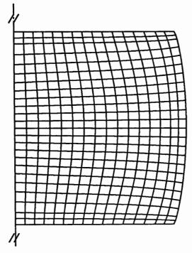
Fig. 7.10 The geometry of the deformed mesh corresponding to the stage in Fig. 7.9
