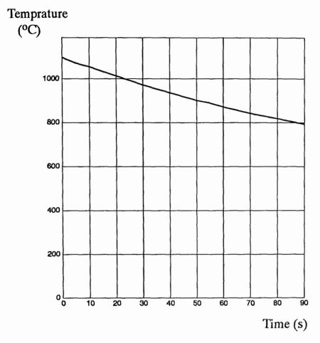
Fig. A.7 Cooling curve for near the surface of the billet Temperature of furnace 1100 °C
