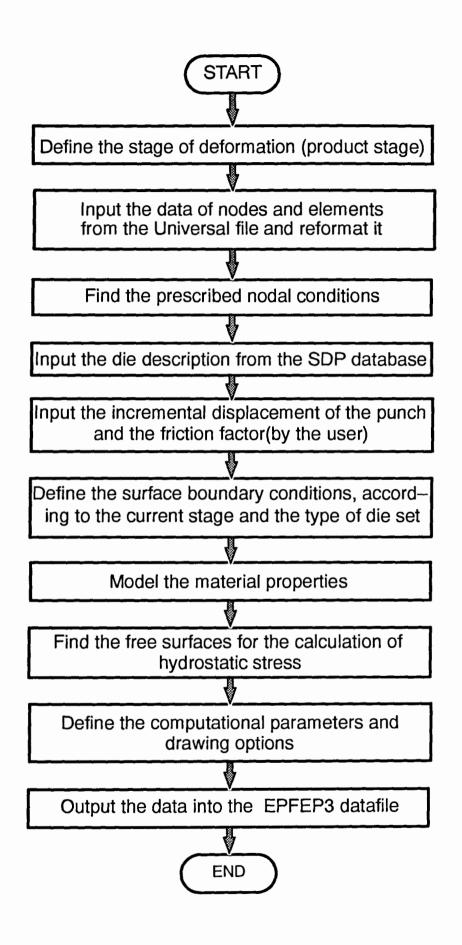
Fig. 4.12 The main actions of producing the datafile
