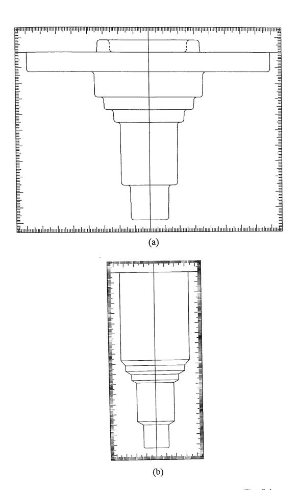
Fig. 8.5 The operational sequences corresponding to Fig. 8.1 (a) Finished part (b) Preform (c) Cheese (d) Billet
