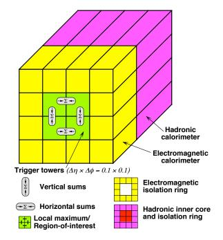
Figure 4.3: An illustration of the L1Calo sliding window algorithm and the various regions which form each window [47].
