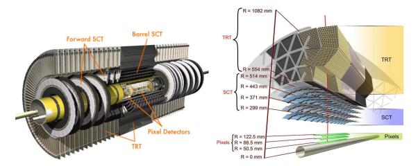
Figure 3.4: A cut away of the Inner Detector layers [34].
