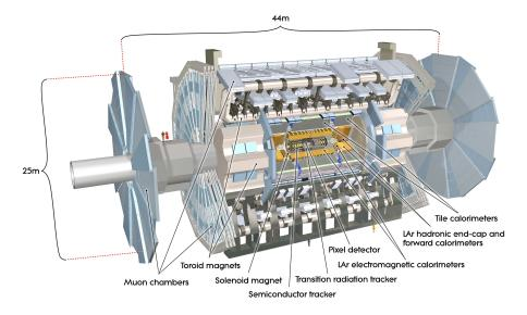
Figure 3.3: A cut-away schematic diagram of the ATLAS detector showing the various subcomponents which make up the detector as a whole [34].
