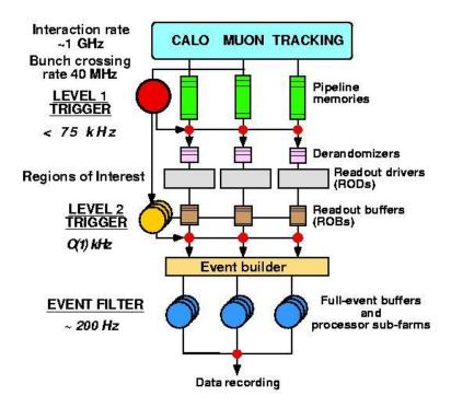
Figure 3.9: A pictorial representation of the three trigger levels used at ATLAS [47].
