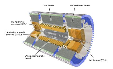
Figure 3.5: A computer generated image of the ATLAS calorimeter system [34].
