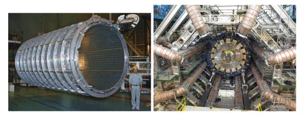
Figure 3.8: An illustration of the barrel solenoid (left) and toroids (right) used at ATLAS [34].
