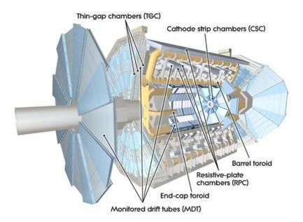
Figure 3.7: An illustration of the muon spectrometer systems surrounding the AT-LAS detector [34].
