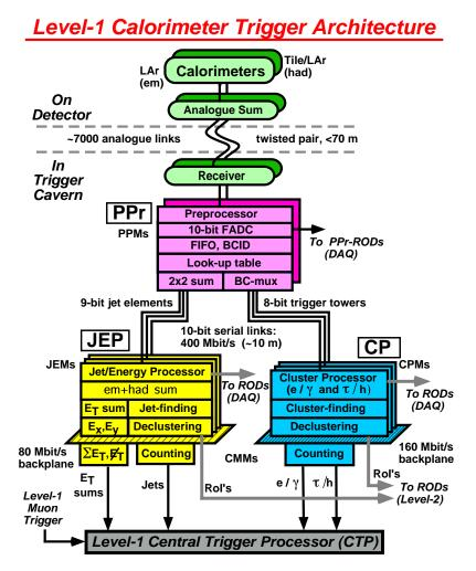
Figure 4.2: A diagram illustrating the various levels of the L1Calo Trigger [35].
