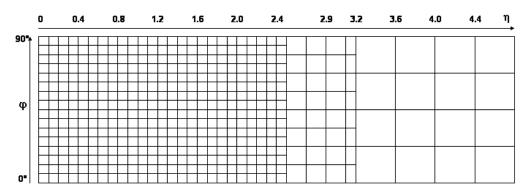
Figure 4.1: An illustration of how the trigger tower granularities vary as a function of their position in their detector [47].
