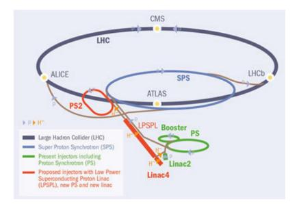
Figure 3.2: A pictorial representation of the injection system used to accelerate protons to high energies at the LHC [40].
