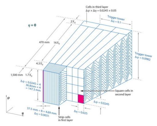
Figure 3.6: An illustration of the liquid argon EM Calorimeter "accordion" structure [34].
