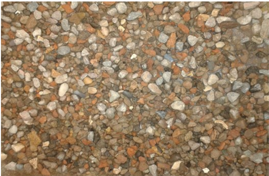
Figure 5: Recycled coarse aggregate (Supplied by Coleman & co. maximum size 10mm)
