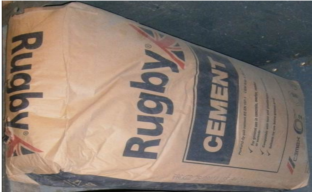
Figure 1: Portland-pulverised fly ash Cement [CEM II/B-V 32,5N]
