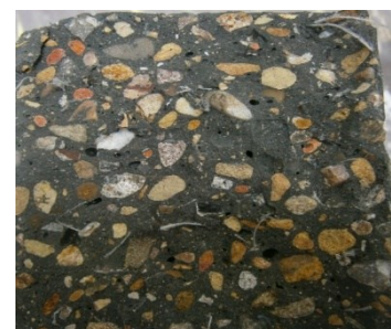
Figure 104. Failure patterns of cube specimens at 28-days compression test (100% RCA)
