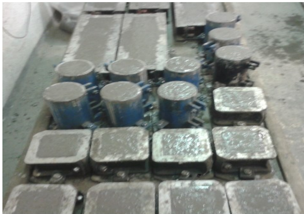
Figure 8: A Concrete moulds conforming to (BS-EN-12390-1, 2012)
