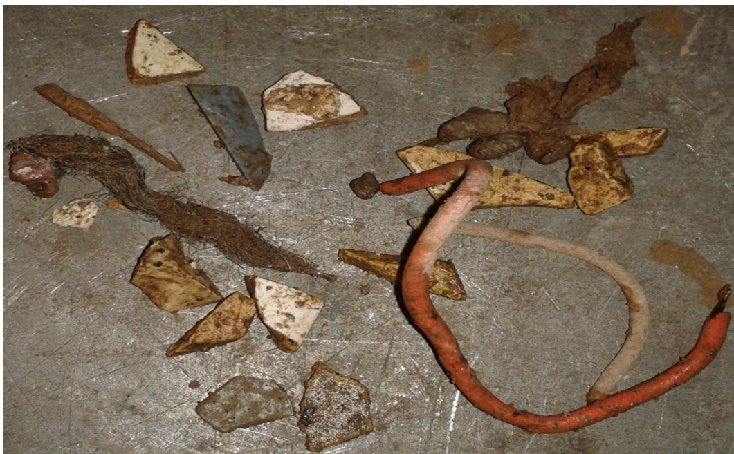
Figure 20: Some impurities found in recycled coarse aggregate
