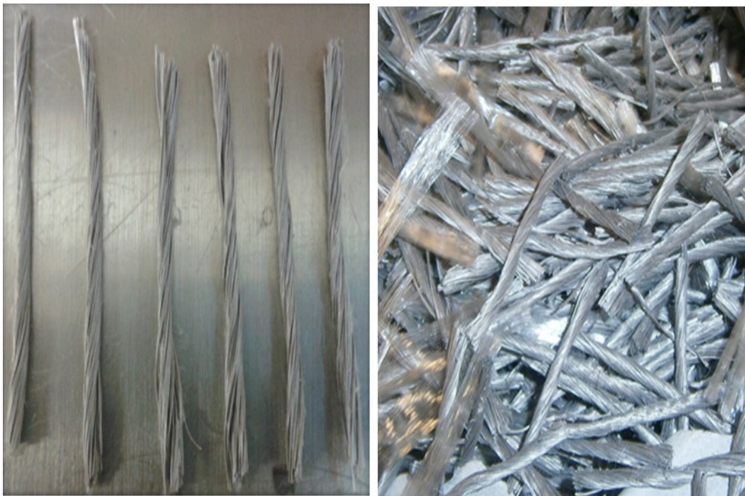
Figure 6: 54mm Forta-Ferro synthetic macro fibre
