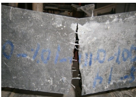
Figure 104. Failure patterns of cube specimens at 28-days compression test (100% RCA)
