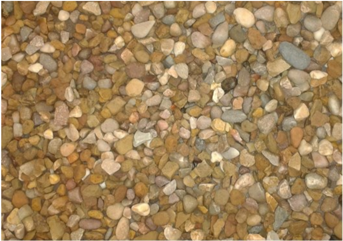
Figure 3: Natural coarse aggregate (Crushed gravel with maximum size 10mm)
