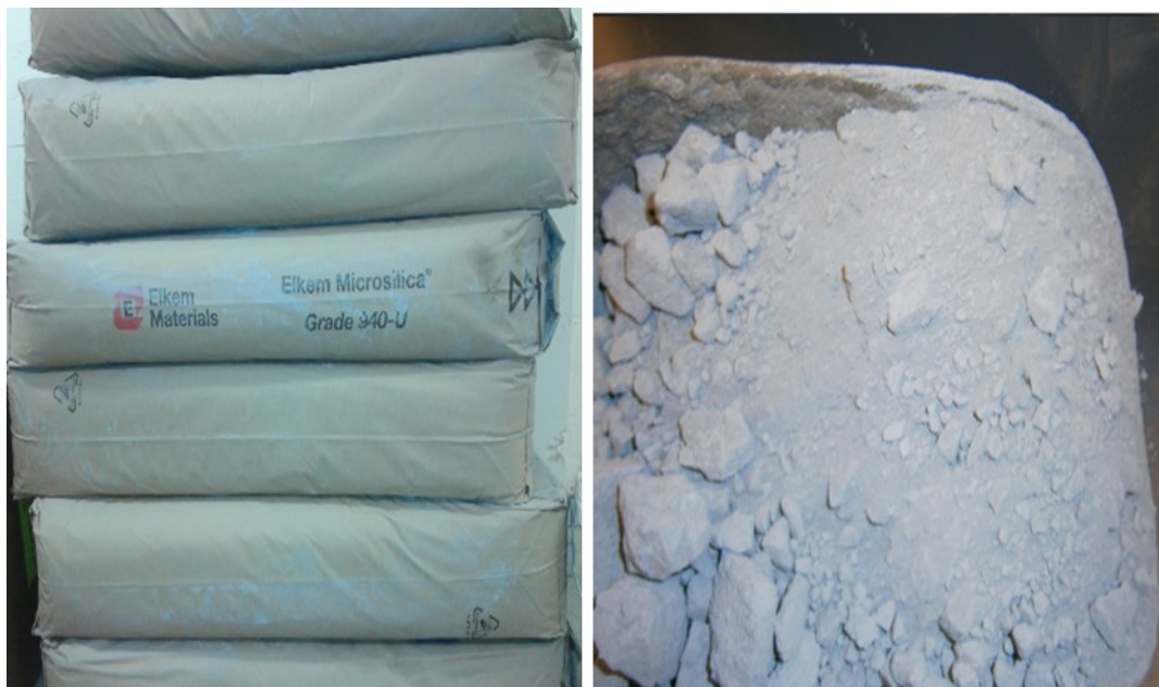
Figure 2: Grade 940-U Microsilica Supplied by Elkem
