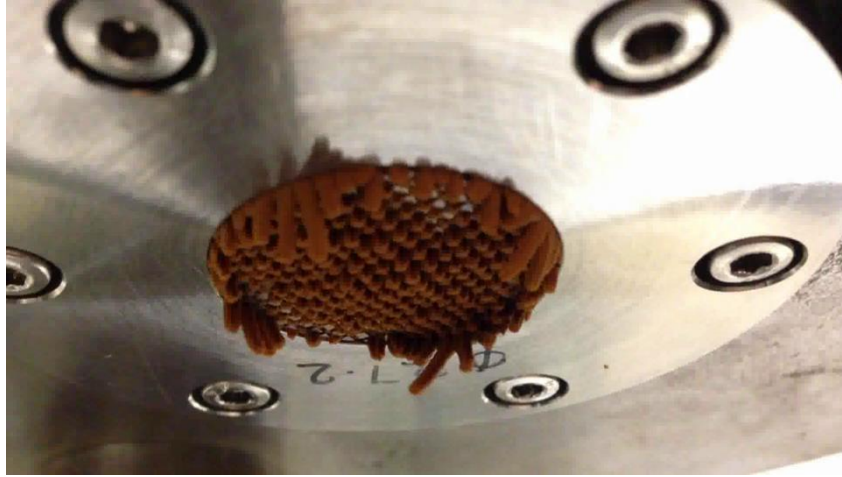
Figure 5.28 – Extrusion profile of reformulated paste
