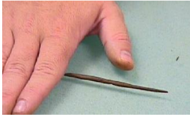
Figure 2.10- Rolling a clay body to measure plastic limit [4]
