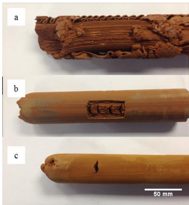
Figure 5.1 - Green monoliths showing different types of extrusion defect
