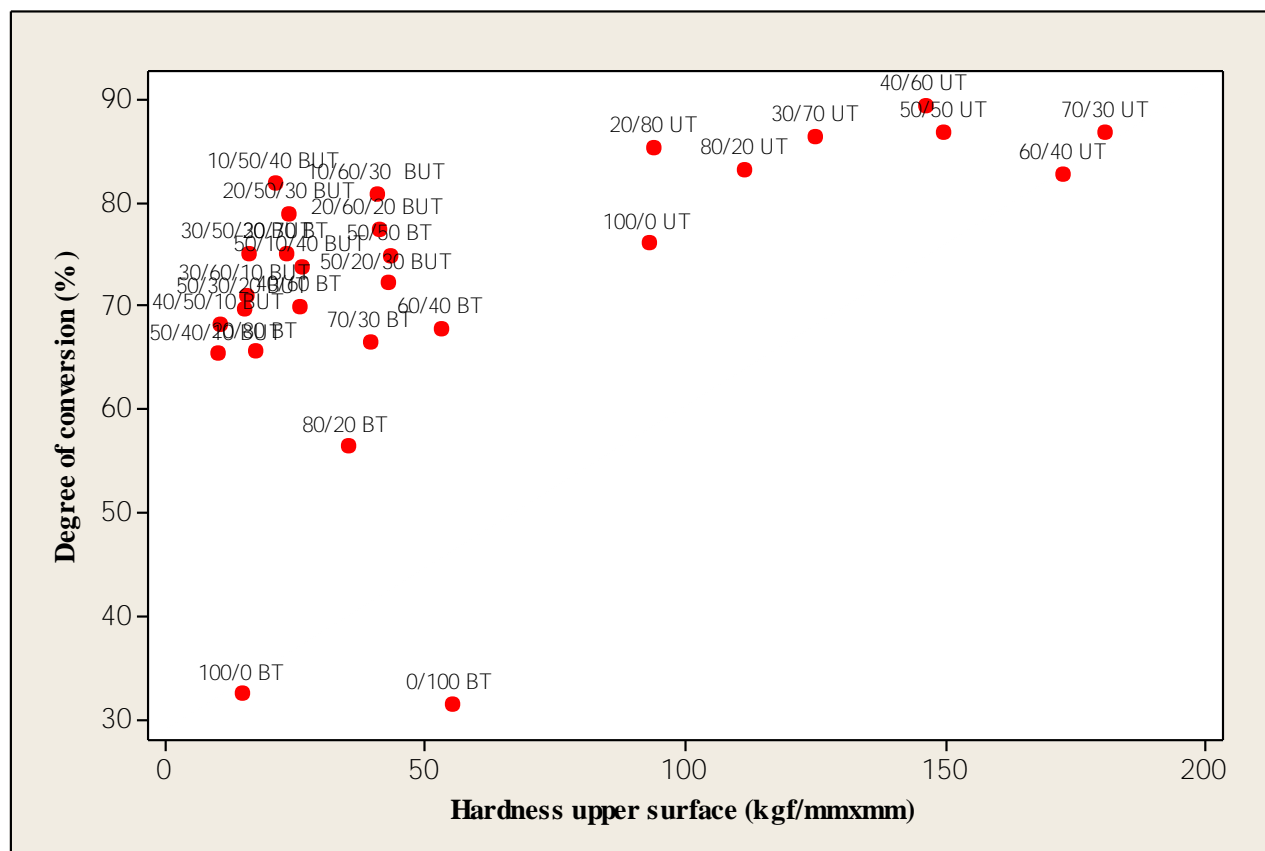
Figure 3.8 Pearson correlation between the degree of conversion and hardness values of unfilled resin systems containing bisGMA/TEGDMA (BT), UDMA/TEGDMA (UT), or bisGMA/UDMA/TEGDMA (BUT). Unfilled resin system percentage inclusions are shown within labels. There was a strong positive correlation between the degree of conversion and hardness values of unfilled resin systems containing 60/40 UDMA/TEGDMA ( r=0.870 ).
