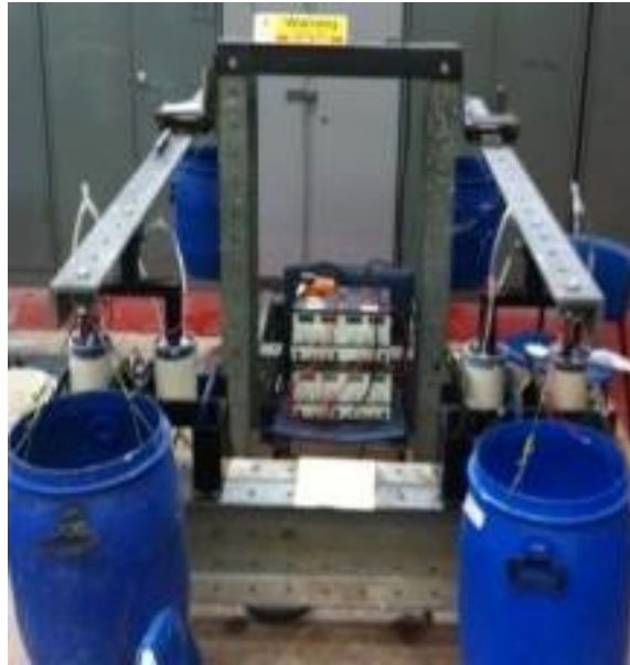
Figure 3.16 Consolidation equipment showing the sample location and the loading mechanism using water tanks
