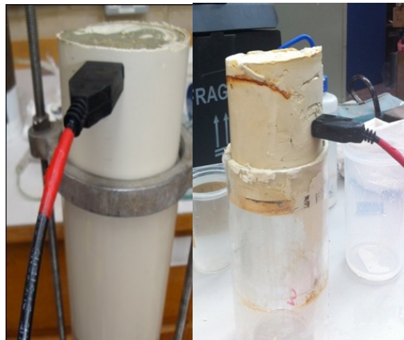
Figure 3.28 TDR probe inserted into a clay sample
