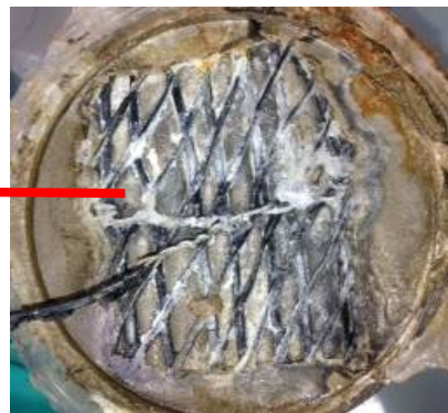
Figure 5.7 Cathode section of Oxford Clay 3-months sample
