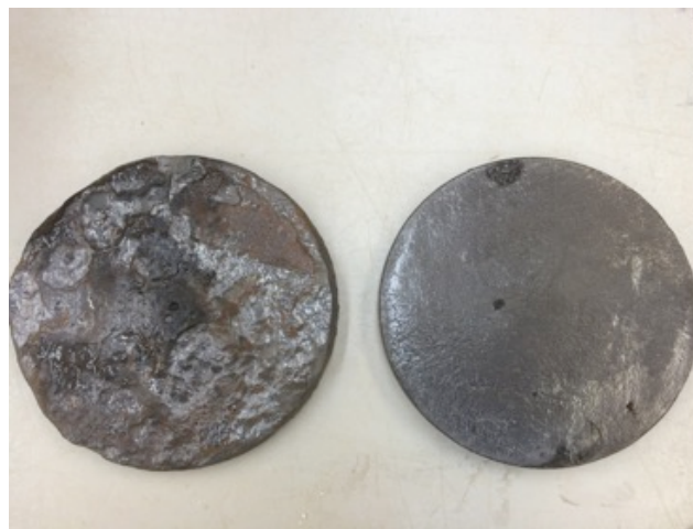
Figure 5.26 Cast iron discs used for Oxford Clay (left side) and Kaolin Clay (right side)
