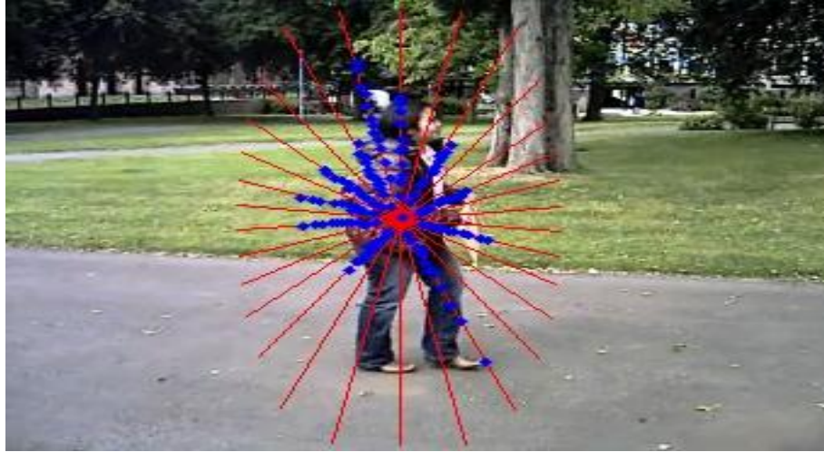
Fig. 6.1. Set of search paths, shown in red, radiating from the central cue point with a set of key points on few search paths, shown in blue, on each search line.
