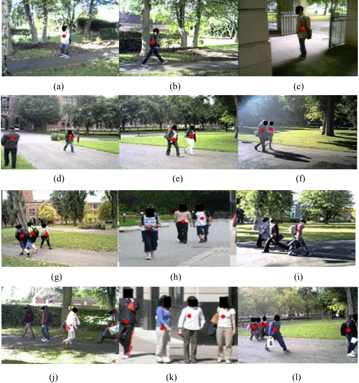
Fig. 7.3. Cue detection for pedestrians with various degrees of crowding and in various poses: (a), (b) and (c) pedestrians alone; (d) two pedestrians at a distance; (e) two relatively close pedestrians; (f) partial occlusion between two pedestrians; (g), (h) and (i) show groups of three pedestrians; (j) and (k) a group of four well spaced pedestrians and (l) a group of five pedestrians in a crowded scene with partial occlusion.
