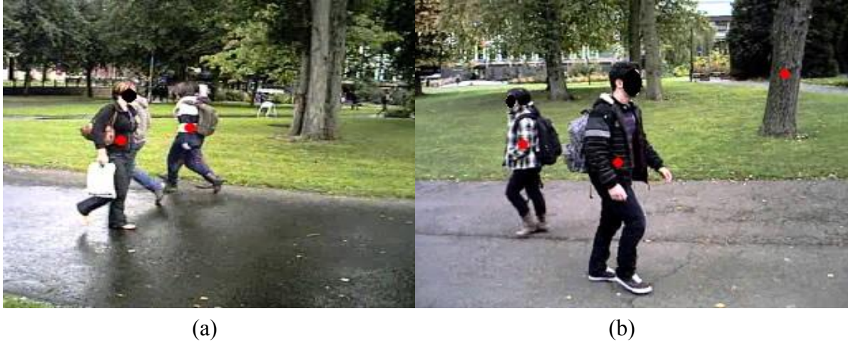
Fig. 7.12. Failure of cue detection: (a) two almost completely occluded pedestrians out of four are not detected and (b) a tree is incorrectly detected.
