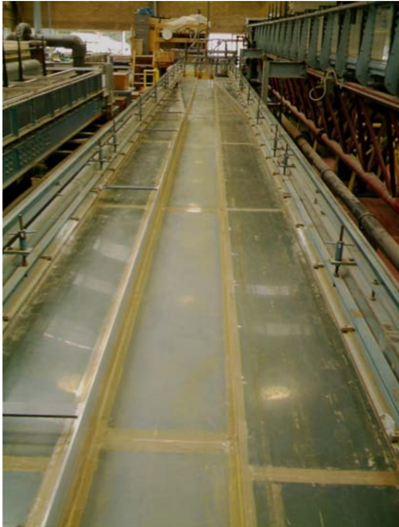
Figure 6.4 -General view of Birmingham flume with skewed floodplains looking downstream
