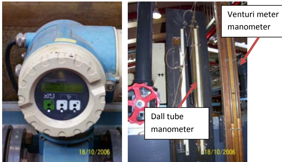
Figure 6.7 a & b -View of the electro-magnetic flow meter, Dall tube and Venturi meter
