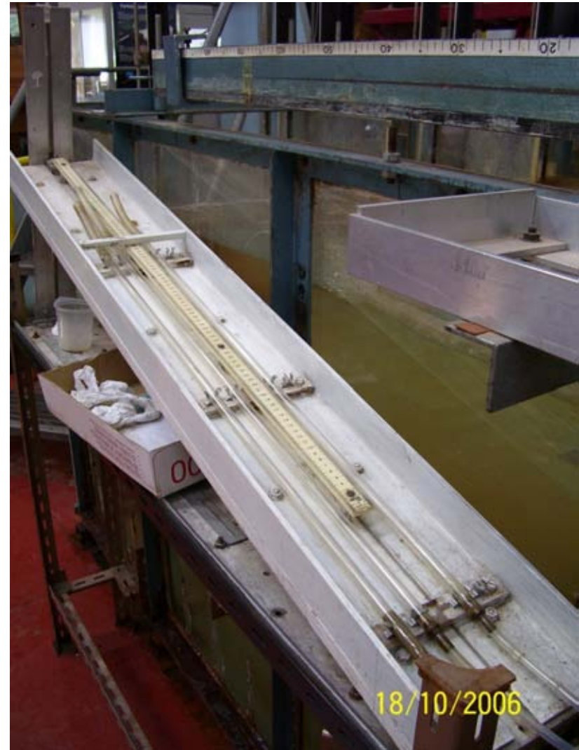
Figure 6.13 -Inclined manometers for boundary shear stress measurements
