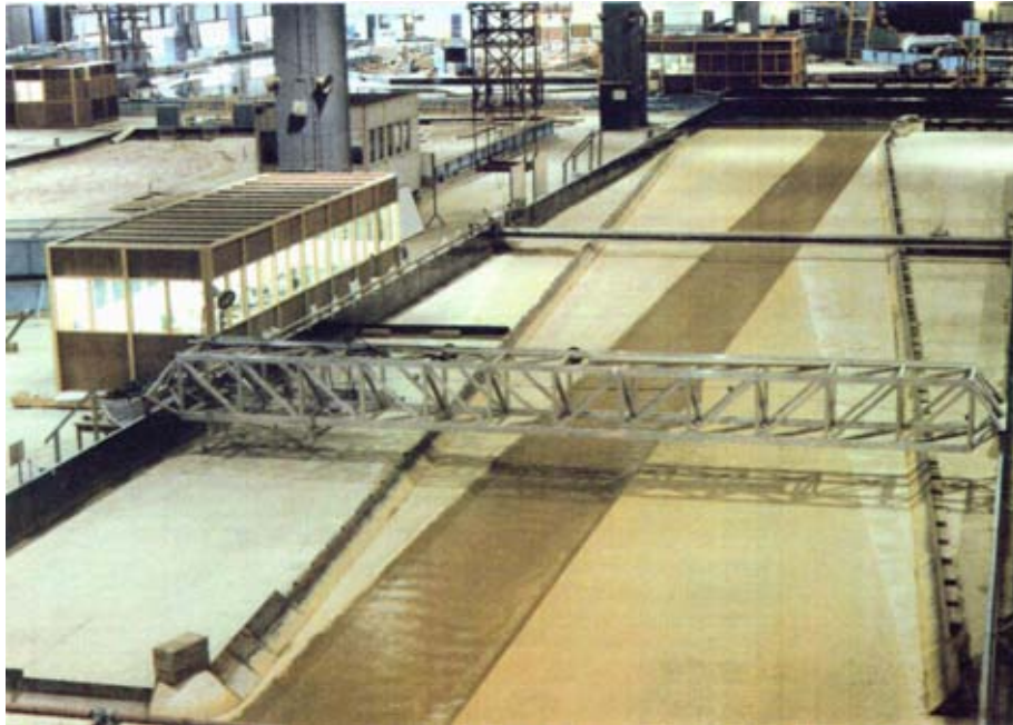
Figure 7.1 -Photograph of FCF skewed channel geometry for skew angle, \theta=5.1^\circ
