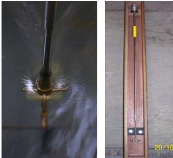
Figure 6.11a & b -Novar Nixon miniature propeller current meter for velocity measurements
