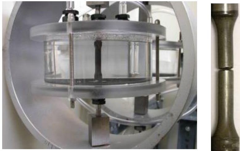
Figure 2.35 NACE TM0177-Method A Standard Tensile Test (proof-ring).
