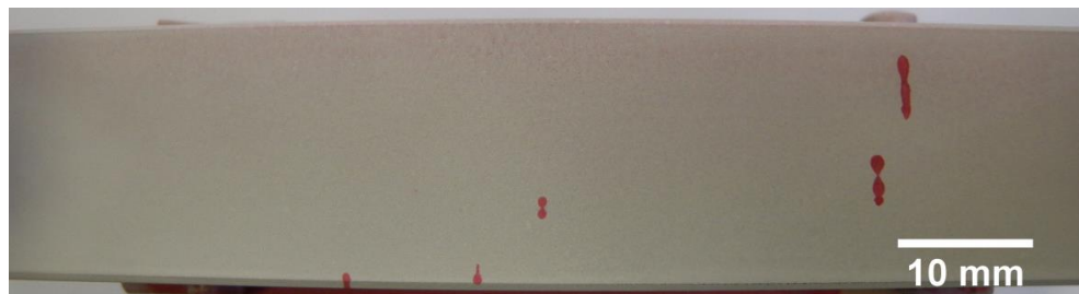
Figure 6.4 Cracking on the fully-machined specimen P8 (PW, 69 mbar H 2 S, 5°C)
