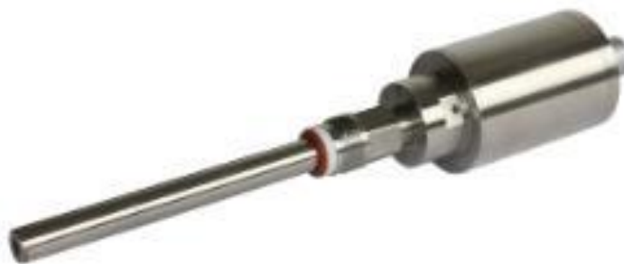
Figure 4.7 Hach-Lange type M1100 luminescence dissolved oxygen sensor
