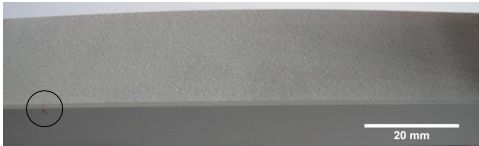
Figure 6.2 Single edge crack on as-received specimen P1 (PW, 69 mbar H 2 S, 24°C)
