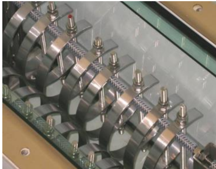
Figure 2.37 NACE TM0177-Method C Standard C-Ring Test.
