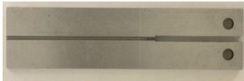
Figure 2.40 NACE TM0177-Method D Standard Double-Cantilever-Beam test specimen.
