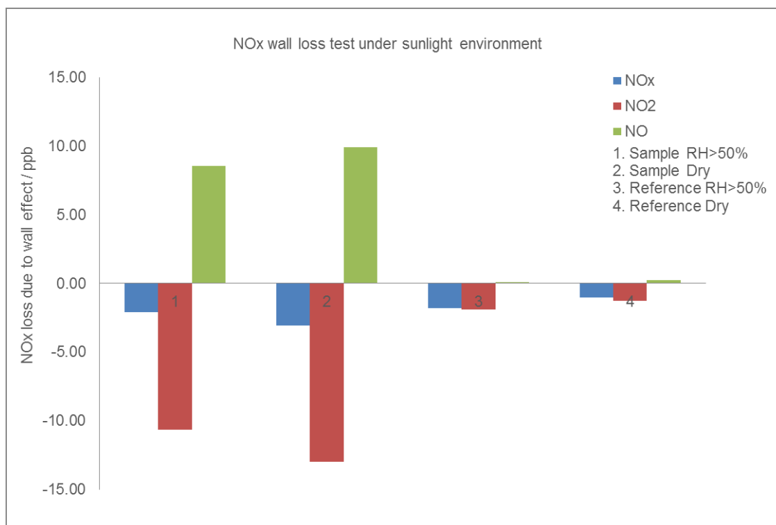
Figures 3.12. Measured NO x loss values (in unit of ppb) due to reactor wall effects, as a function of flow RH under sunlit conditions. Different reactor and RH combinations are mentioned in the figure legend. The synthetic NO 2 addition was manually set to 65 ppb during this experiment.
