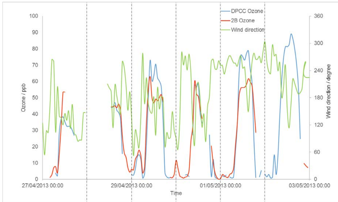
Figure 6.11. Comparison between ozone levels measured at the DPCC Delhi International Airport monitoring station, and those measured using the University of Birmingham 2B monitor at TERI University during TSMT period (left axis). The wind direction during this period is shown on the right axis.
