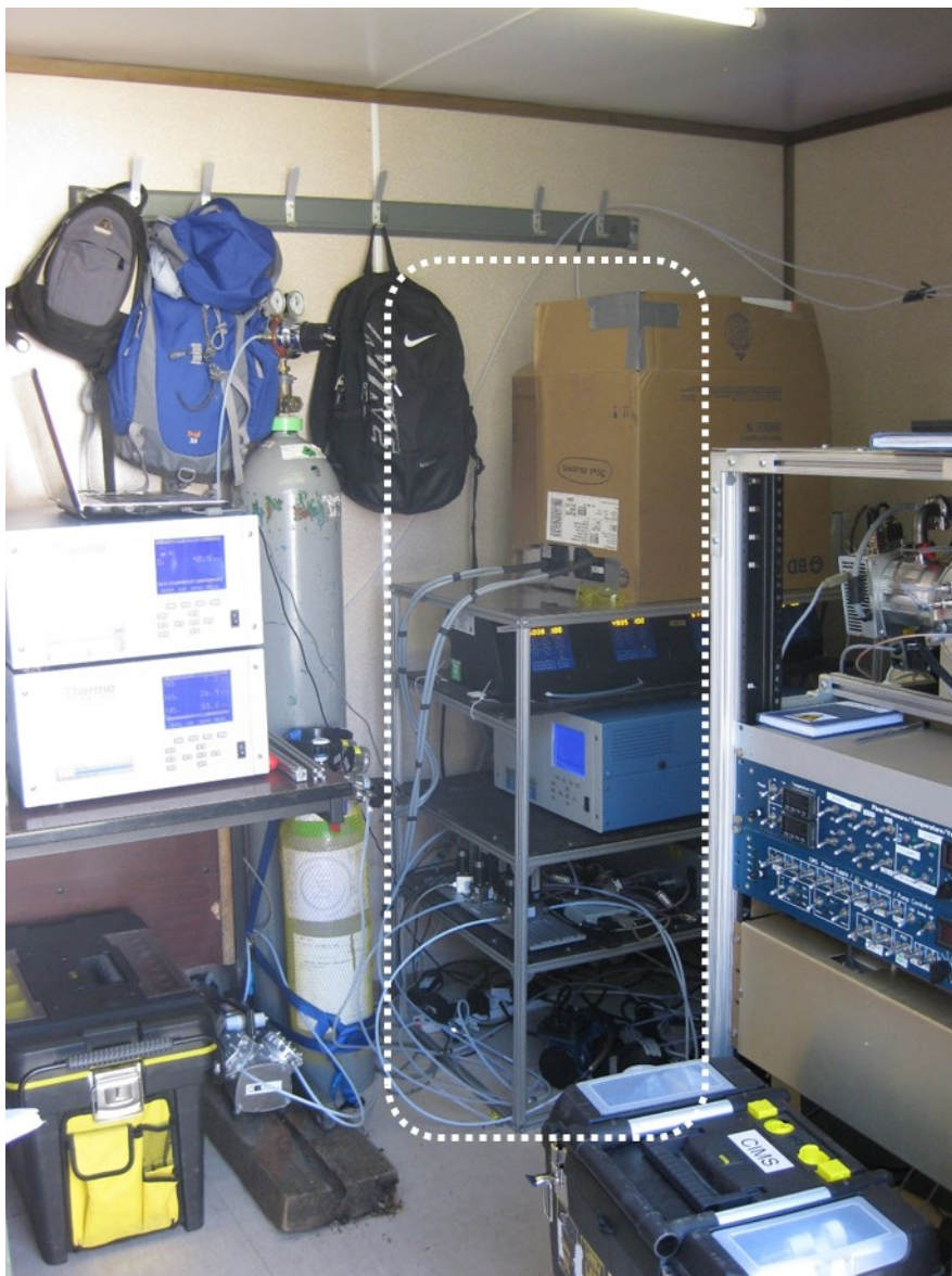
Figure 2.2. OPR core unit (OPR system components without the dual sampling reactors) during ClearLo London summer IOP (located in white circle area).
