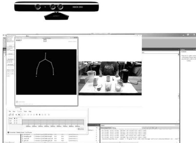
Figure 3.3: Kinect TM user interface with skeleton view of arms and hands [33]
