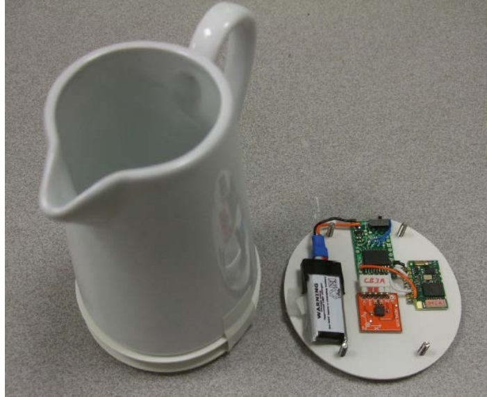
Figure 3.2: A jug fitted with a CogWatch Instrumented Coaster (CIC) and an ‘open’ CIC, showing the accelerometer, PIC microcontroller, Bluetooth module and battery [33]
