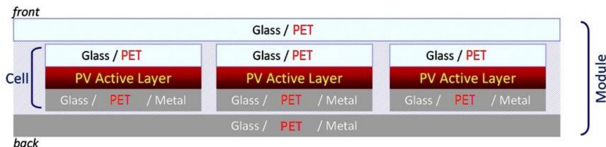
Figure 1.1: Simplified schematic layout of a PV module
