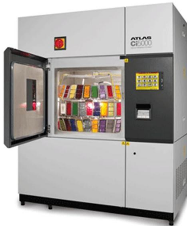
Figure 3.8: ATLAS Ci5000 Weather-o-meter in operation at DTF (Plasticker, 2012)
