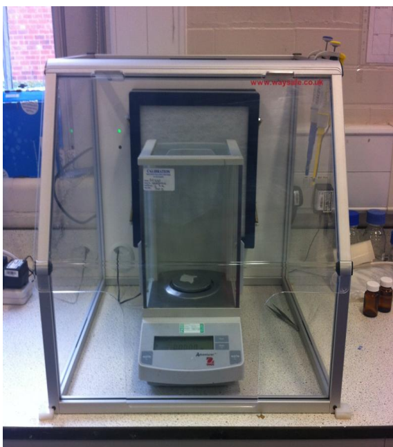
Figure 3-7 Waysafe 3 glove box and Ohaus Adventurer analytical balance.
