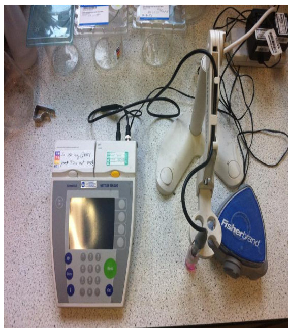
Figure 3-8 Mettler Toledo SevenMulti pH meter and Fisherbrand magnetic stirrer.
