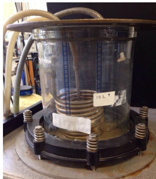
Figure 3-5 Glass reservoir (Break vessel): made from QVF glassware (0.015 – 0.018) m 3
