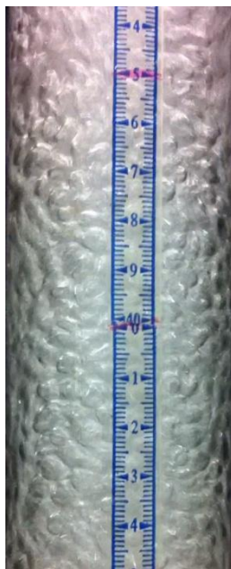
Figure 3-12 Bubble size measurements method by visual analysis in the vicinity of the column wall using reference tape (scale in mm) attached to outside of the DGCR column.
