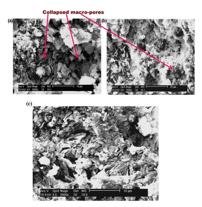
Figure 5.3: SEM microstructure of unwashed natural zeolite thermally pre – treated in a muffle furnace for 30 minutes at (a, b) 400 °C (c) 200 °C.
