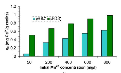
Figure 6.11: Amount of exchangeable  $Ca^{2+}$  ions in solution at equilibrium, for different initial manganese concentrations.
