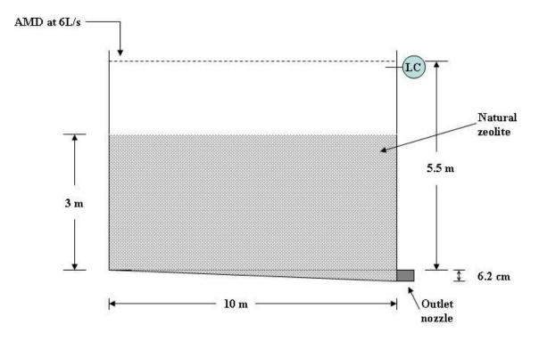
Figure 9.3: Sketch of the proposed reactor for the passive treatment of Wheal Jane AMD.
