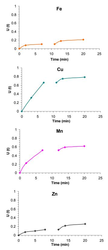
Figure 7.15: Interruption tests on the removal of heavy metals from solution by natural zeolite (3.7g natural zeolite, 100 ml single component solution, pH 3.5).
