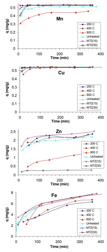
Figure 7.7: Comparison of natural and thermally pre – treated natural zeolite, 3.7 g mixed with 100ml single component solutions at pH 3.5.
