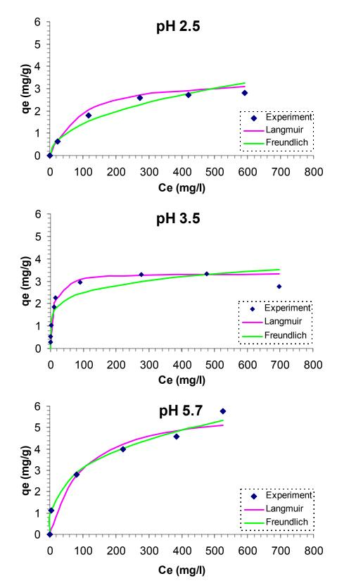
Figure 6.1: Equilibrium isotherms for the removal of copper from solution.
