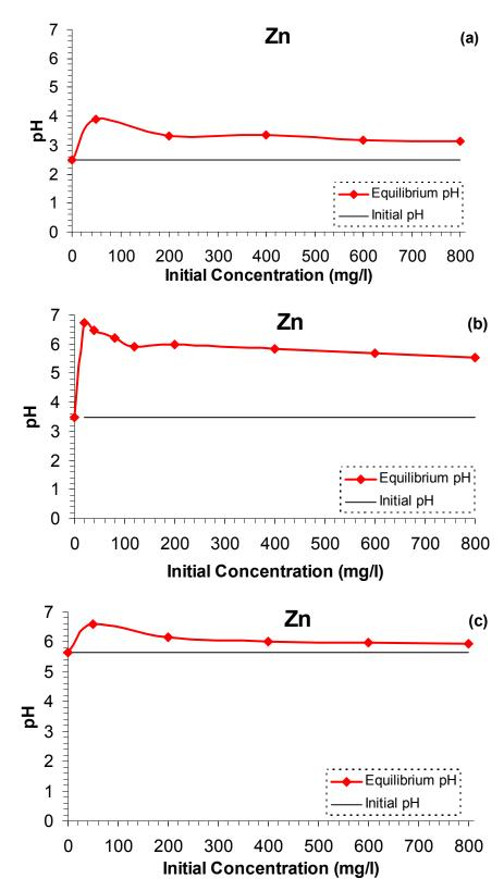
Figure 6.5: Change in equilibrium pH with respect to various initial zinc concentrations. The initial solutions where at different pH values, which are: (a) 2.5, (b) 3.5 and, (c)  $5.7 \pm 0.1$ .
