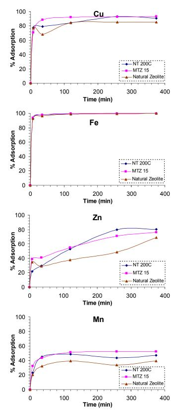
Figure 9.1: Effect of thermally pre-treating natural zeolite on its capacity to remove heavy metals from Wheal Jane mine AMD.
