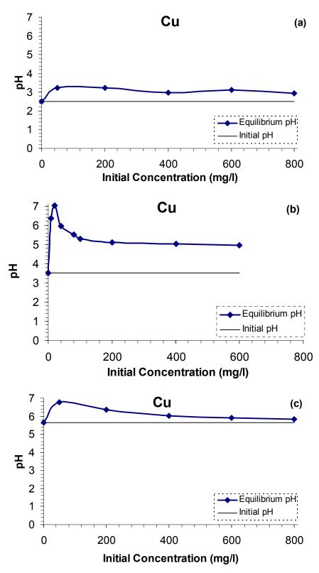
Figure 6.2: Equilibrium pH change with respect to various initial copper concentrations. The initial solutions where at different pH values, (a) 2.5, (b) 3.5 and, (c) 5.7. Error in pH reading is  $\pm 0.1$ .
