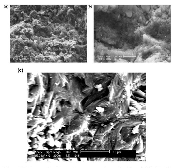
Figure 5.5: Micrographs of thermally pre – treated natural zeolite at *i*. 800 °C (a, b) and *ii*. 30 minute exposure to microwave energy at 950 W, (c).
