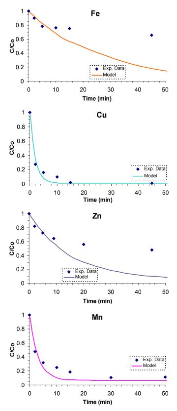
Figure 7.12: Fitting film transfer diffusion control model to the experimental results.
