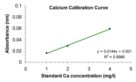
Figure A3: Typical calibration curve for calcium obtained using the AAS.
