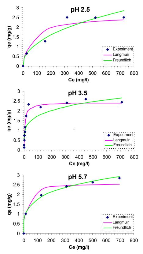
Figure 6.9: Equilibrium isotherms for the removal of manganese from solution by natural zeolite at different initial solution pH levels.
