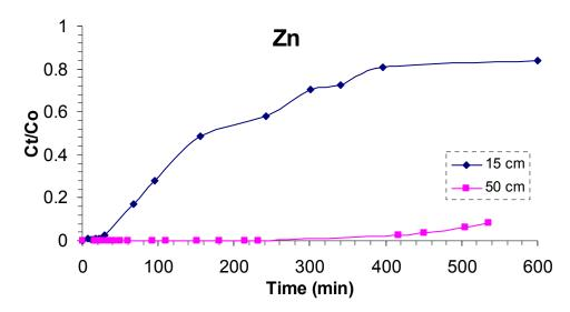
Figure 8.6: Effect of bed height on the adsorption of zinc by natural zeolite;  $C_0 = 120$  mg/l.
