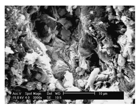
Figure 5.1: SEM micrograph of natural zeolite (Clinoptilolite) at a magnification of x3000; the natural zeolite was washed in distilled water.
