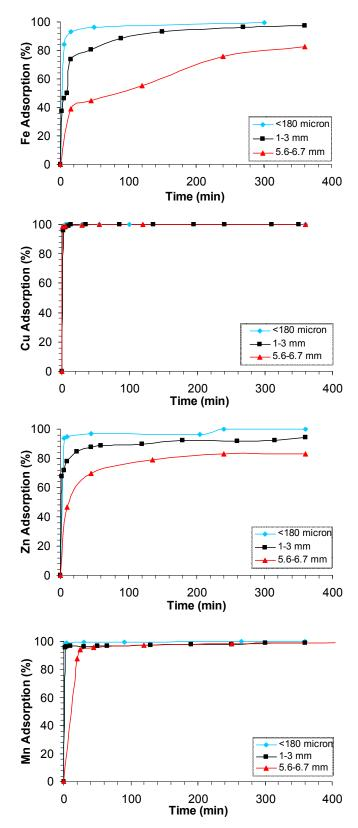
Figure 7.2: Effect of Particle size on the adsorption of iron, copper, zinc and manganese from solution (15 g of zeolite in 100 ml solution; solution pH 3.5).
