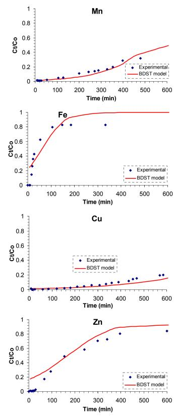
Figure 8.3: Comparison of the BDST model with experimental results, bed height 15 cm, flow rate 20 ml/min and the BDST model was calculated at 30 % breakthrough.
