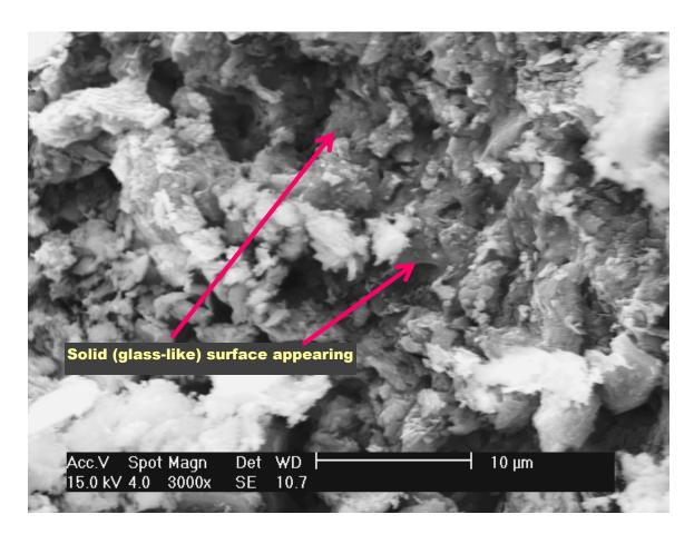
Figure 5.4: SEM microstructure of natural zeolite thermally pre – treated in a microwave for 15 minutes.
