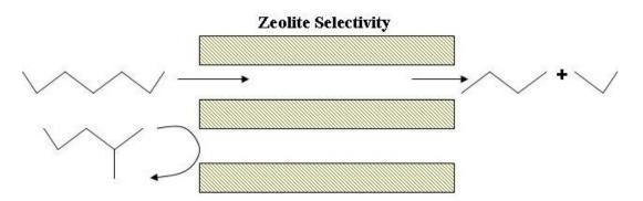
Figure 2.4: Shape selectivity in zeolite channels (Csicsery, 1985).
