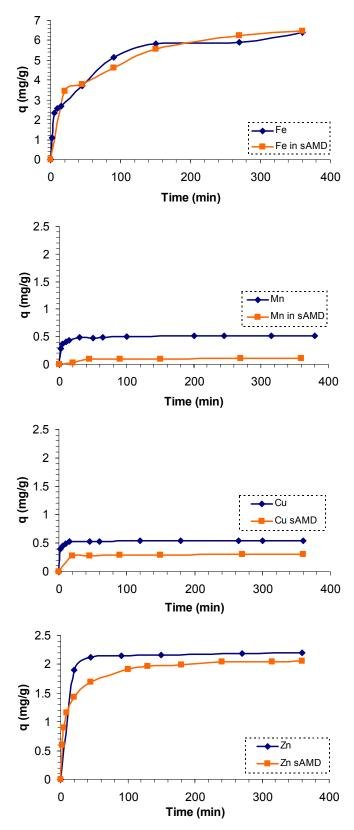
Figure 7.9: Comparison of adsorption capacities from single component solutions and from synthetic acid mine drainage (sAMD).
