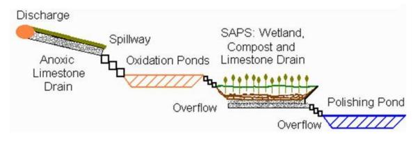
Figure 2.1: An example of a common Passive treatment system (Reprinted from: <a href="http://www.scrip.pa-conservation.org/aboutamd.htm">http://www.scrip.pa-conservation.org/aboutamd.htm</a>).
