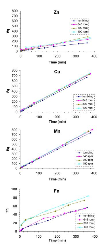
Figure 7.11: Effect of agitation speed on the reaction rate constant.
