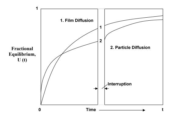
Figure 7.14: The effect of interruption upon the rate of exchange according to controlling diffusion mechanism (schematic) (Harland, 1994).
