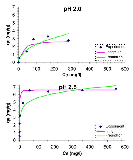
Figure 6.7: Equilibrium isotherms for the removal of iron from solution by natural zeolite at different initial solution pH levels.
