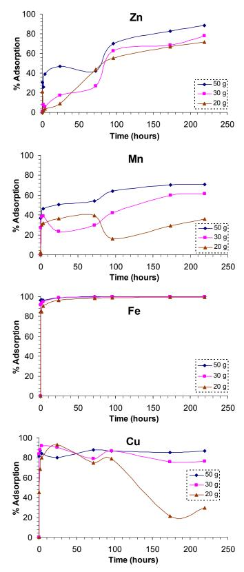
Figure 9.2: Treatment of Wheal Jane mine AMD using natural zeolite (no agitation for about 9 days).
