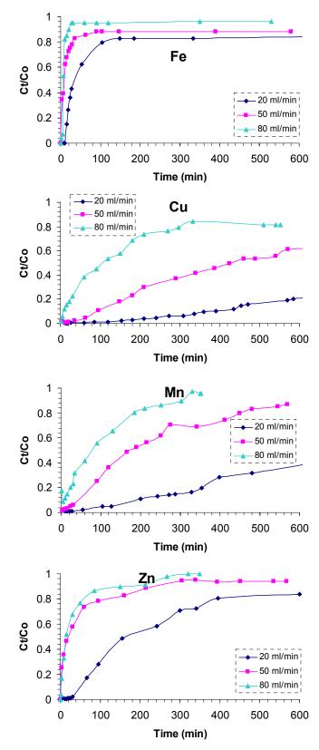
Figure 8.4: Breakthrough curves for the effect of flow rate on the adsorption of heavy metals by natural zeolite.
