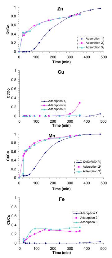
Figure 9.5: Breakthrough curves for the treatment of Wheal Jane AMD; bed height 50 cm and flow rate 20 ml/min.
