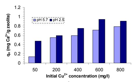
Figure 6.3: Amount of exchangeable  $Ca^{2+}$  ions in solution after equilibrium, at different initial copper concentrations.
