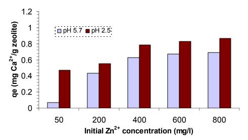
Figure 6.6: Amount of exchangeable  $Ca^{2+}$  ions in solution at equilibrium, for different initial zinc concentrations.
