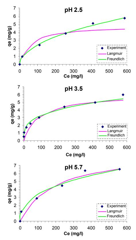
Figure 6.4: Equilibrium isotherms for the removal of zinc from solution by natural zeolite at different initial solution pH levels.
