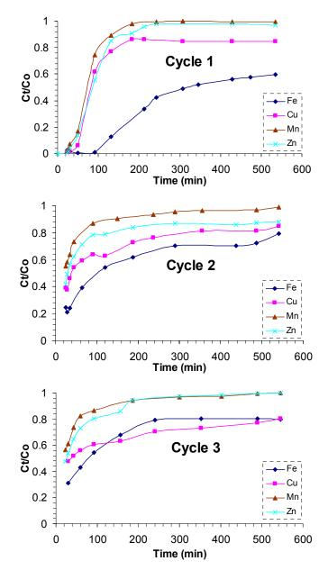
Figure 8.7: Breakthrough curves for the removal/adsorption of heavy metals from synthetic solutions by natural zeolite, bed height 50 cm and flow rate 20 ml/min.
