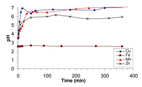
Figure 7.4: Change in solution pH as adsorption of heavy metals proceeds (3.7 g zeolite; 100 ml single component solution; particle size 1 - 3 mm).
