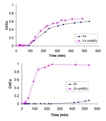
Figure 8.8: Breakthrough curves for the effect of competing cations in the removal of zinc and iron from single component and sAMD solutions; bed height 50 cm, flow rate 20 ml/min.
