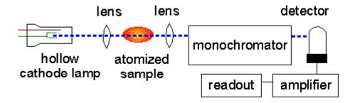
Figure A1: Schematic of atomic absorption spectrometer (Tissue, 1996). [Reprinted from: <u>http://elchem.kaist.ac.kr/vt/chem-ed/spec/atomic/aa.htm</u>].
