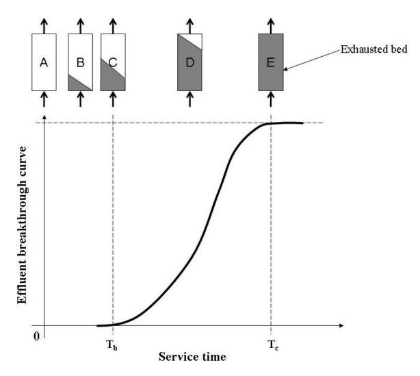
Figure 8.2: Schematic representation of the displacement of the adsorption zone or mass transfer zone and the resulting breakthrough curve (Harland, 1994).
