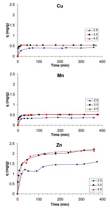
Figure 7.3: Effect of initial solution pH on the adsorption capacity of natural zeolite (3.7 g zeolite; 100 ml single component solution; particle size 1 - 3 mm).
