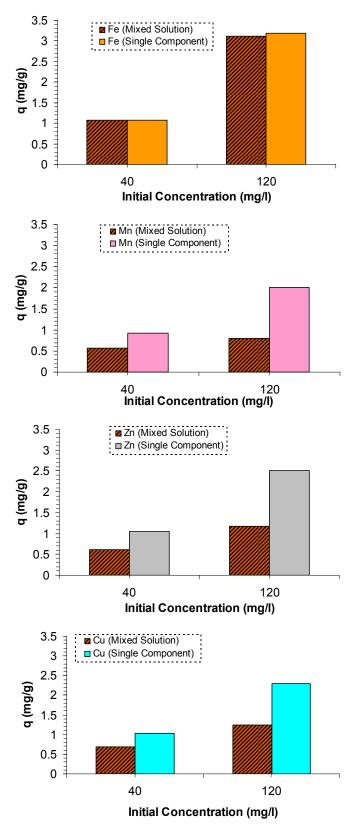
Figure 7.6: Comparison of the adsorption capacity of natural zeolite for iron, manganese, zinc and copper from single and multi – component solutions.
