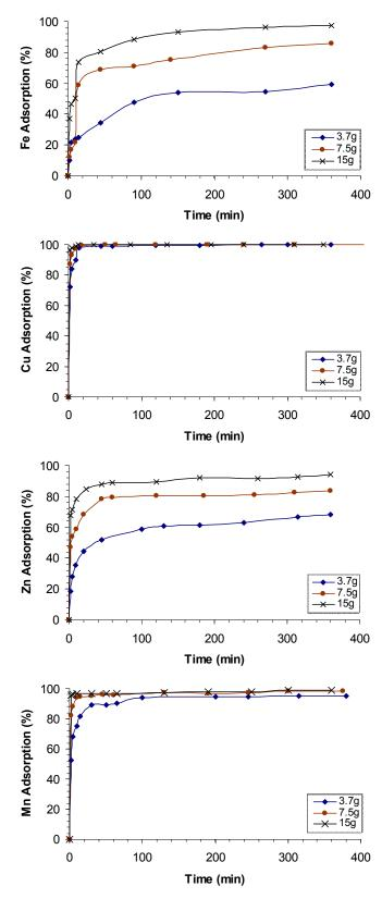
Figure 7.1: The effect of the mass of natural zeolite on the adsorption of iron, copper, zinc and manganese from solution (particle size: 1 - 3 mm; pH: 3.5).
