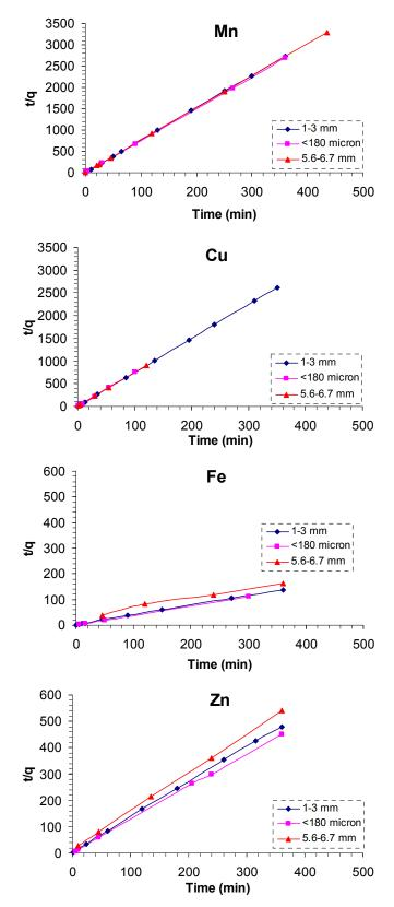
Figure 7.10: Effect of adsorbent particle size on the reaction rate constant.
