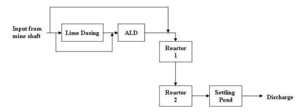
Figure 9.4: Proposed flow diagram for the passive treatment of AMD from Wheal Jane mine.
