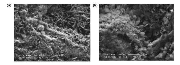
Figure 5.2: SEM micrographs of acid washed natural zeolite (Clinoptilolite) at different magnifications: (a) x 1000 and (b) x 2000.
