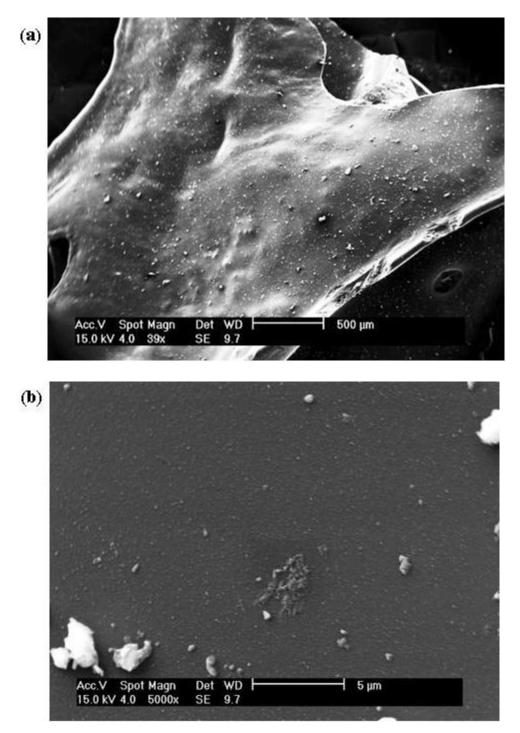
Figure 5.6: SEM microstructure of natural zeolite whose macro – pores have completely collapsed due to thermal runaway, (a) x39, (b) x5000.
