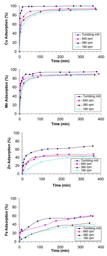
Figure 7.5: Effect of agitation on the adsorption of heavy metals by natural zeolite (3.7 g in 100 ml solution).
