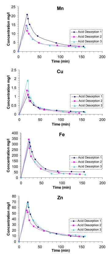
Figure 9.6: Desorption of heavy metals from natural zeolite using 2 % (w/w) sulphuric acid at 40 °C; flow rate 20 ml/min; column bed height 50 cm.
