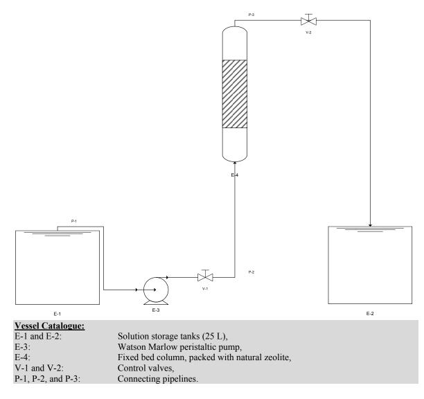
Figure 4.1: Schematic diagram of the column set – up.
