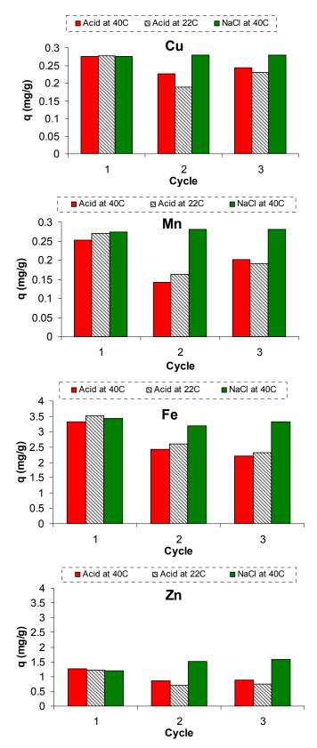
Figure 7.8: Change in the adsorption capacity of natural zeolite due to regeneration.
