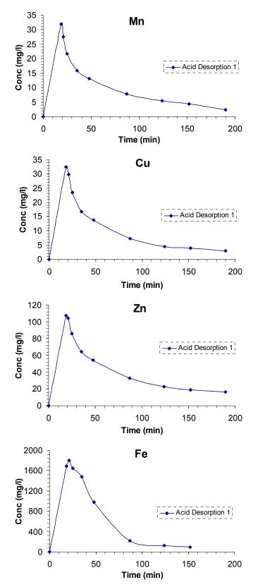
Figure 8.9: Desorption of heavy metals from natural zeolite; column bed height 50 cm, cycle 1.
