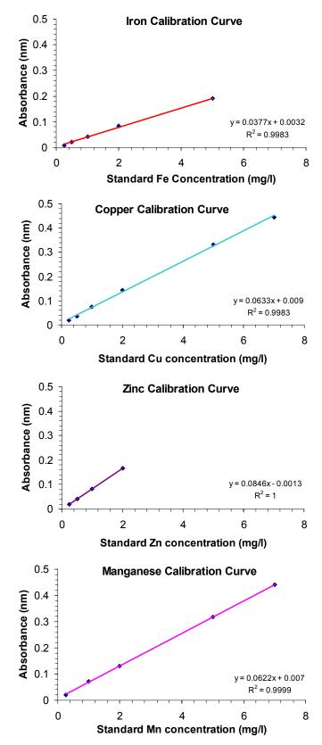
Figure A2: Typical calibration curves for iron, copper, zinc and manganese obtained using the AAS.
