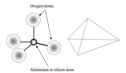
Figure 2.2: Representation of [SiO<sub>4</sub>]<sup>4-</sup> or [AlO<sub>4</sub>]<sup>5-</sup> tetrahedral (Dyer, 1988).
