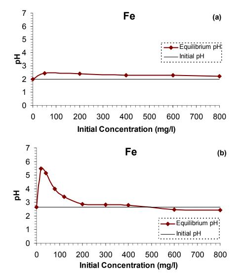
Figure 6.8: Equilibrium pH change with respect to different initial iron concentrations. The initial solutions where at different pH values, which are: (a) 2.0 and, (b)  $2.5 \pm 0.1$ .
