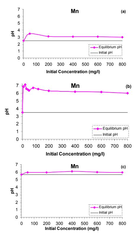
Figure 6.10: Equilibrium pH change with respect to various initial manganese concentrations. The initial solutions were at pH: (a) 2.5, (b) 3.5 and, (c)  $5.7 \pm 0.1$ .
