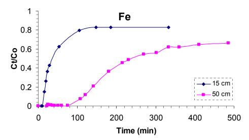
Figure 8.5: Effect of bed height on the adsorption of iron by natural zeolite;  $C_0 = 400 \text{ mg/l.}$
