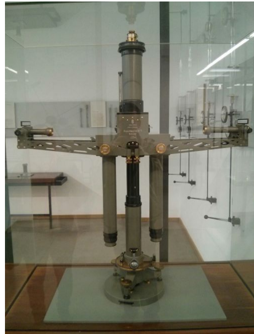
(b) Eötvös pendulum showcased in the Deutsches Museum (German Museum) in Munich. The device features two tubes in which both, the sample and the reference mass are suspended.
