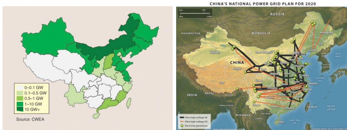
Figure 1-5 (left) Distribution of wind resource in China; (right) China power grid plan for 2020.
