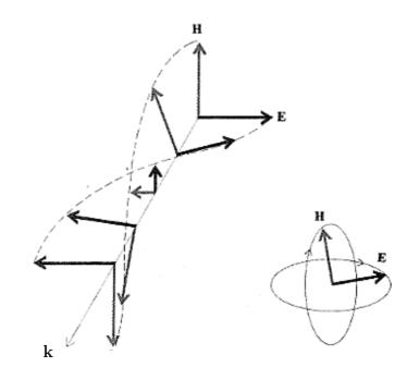
Figure 2.2: Visualisation of elliptically polarised light (image from [43])
