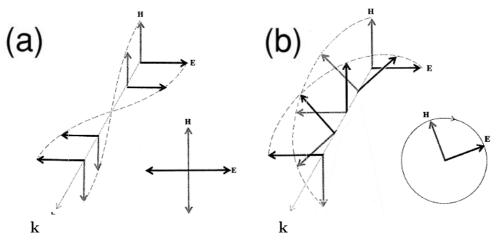
Figure 2.1: Visualisation of both Linearly (a) and Circularly (b) polarised light (images from [43])
