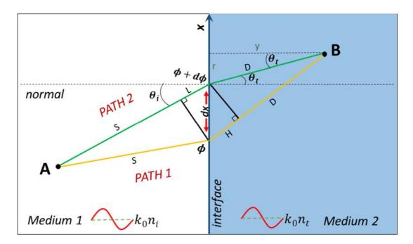
Figure 2.9: Geometric representation of Fermat's 'Principle of Least Optical Path' for deriving Generalised Snell's Law
