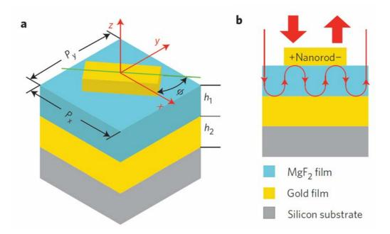
Figure 6.1: Schematic diagram of the unit-cell element used for high polarisation conversion [69]
