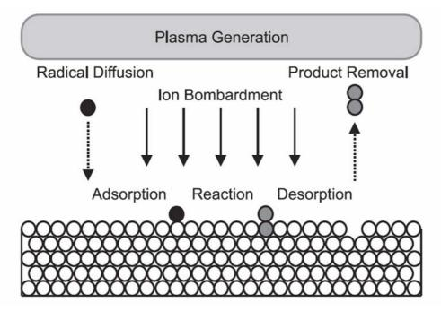
Figure 3.7: Schematic representation of the etching methods present in a RIE process [74]
