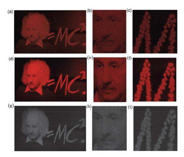
Figure 6.6: Simulated and optical verification of the holographic image at different wavelengths [69]
