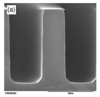
Figure 3.8: DRIE etch profile of silicon with SF6 when using Oxygen as a passivation/inhibitor gas to obtain vertical sidewalls [74]
