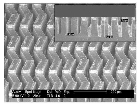
Figure 4.5: SEM Image of etched Silicon Herringbone metasurface
