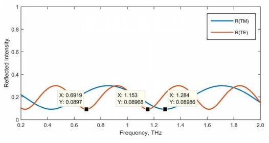
Figure 4.1: Reflectivity of Form-Birefringent Gratings without angular disparity and without silicon step
