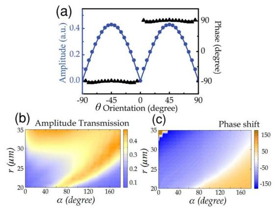
Figure 5.3: Simulated transmission amplitude and phase response of a fixed-geometry C-shaped antenna array [118] and varying-geometry C-antennas [83]
