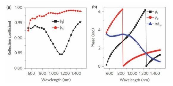
Figure 6.2: Simulated Amplitude and Phase responses of a metasurface array with fixed rotation angle [69]
