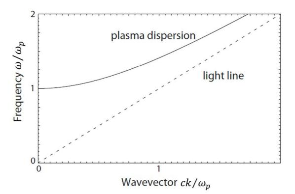
Figure 2.4: Dispersion relation of metals with a free-electron gas/plasma described by the Drude Model [47]
