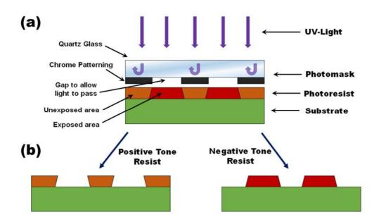
Figure 3.2: Schematic of Photolithographic process
