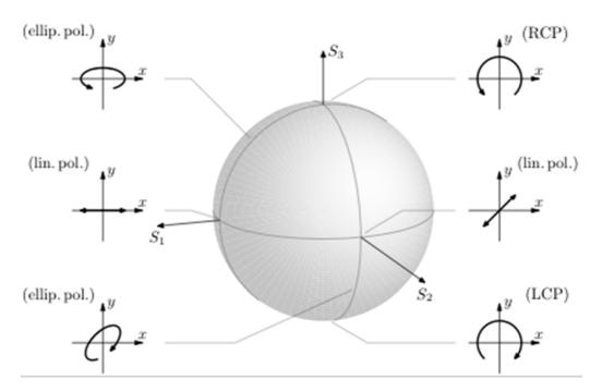
Figure 2.6: Visual illustration of the Poincaré Sphere for representing polarisation states of light [52]
