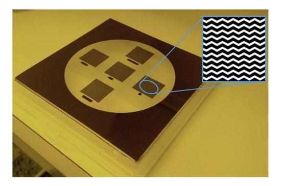
Figure 3.5: Photograph of a photomask designed for use with the Karl Suss MJB-3 Mask Aligner
