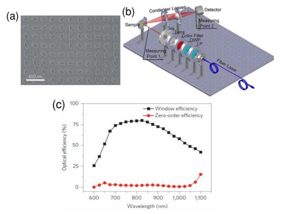
Figure 6.5: Scanning electron microscopy image, experimental optical setup and results for optical efficiency [69]
