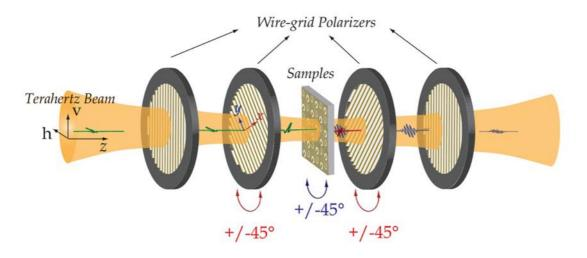
Figure 3.18: Schematic diagram of a THz-TDS experimental setup (Image from [84])
