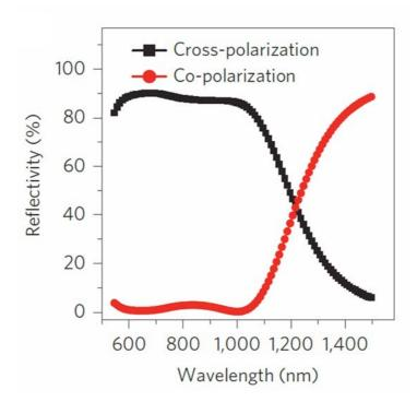
Figure 6.3: Simulated cross-polarisation and co-polarisation with normal light incidence for design in Fig. 5.1. [69]
