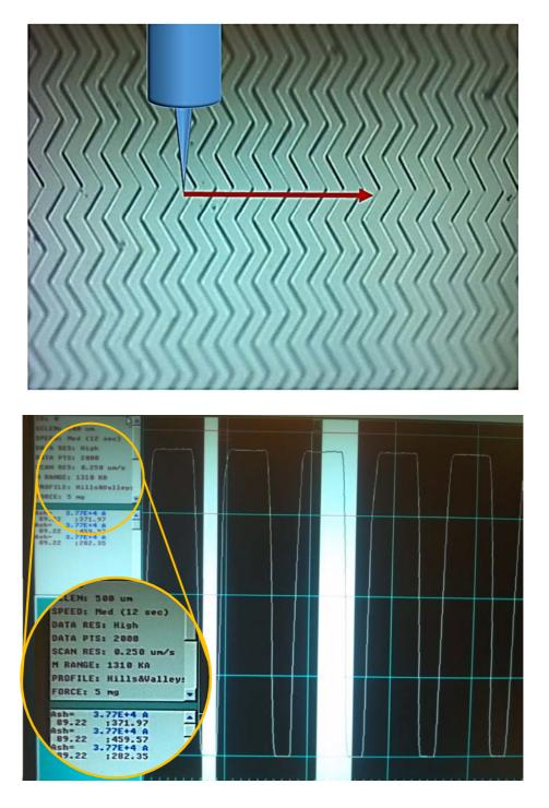
Figure 3.16: Camera image and corresponding surface profile of a section of etched herringbone pattern
