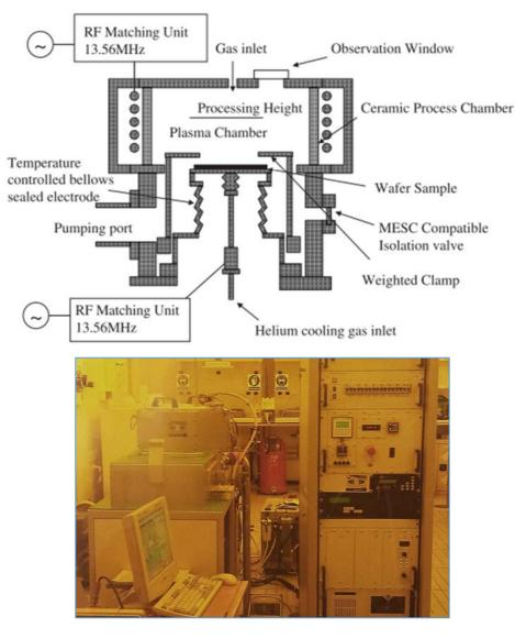
Figure 3.6: Schematic and photograph of an STS ICP DRIE etcher [72]
