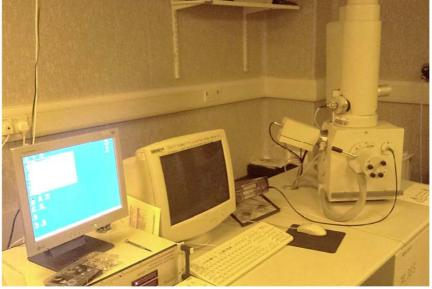
Figure 3.14: Schematic diagram and photograph of a Scanning Electron Microscope
