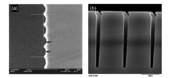
Figure 3.10: Scalloping effect of the sidewalls in the Bosch Process [79] and the narrowing of the trench with increasing depth [74]
