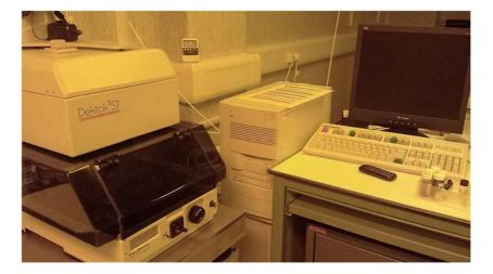
Figure 3.15: Dektak<sup>3</sup> ST Surface Profilometer
