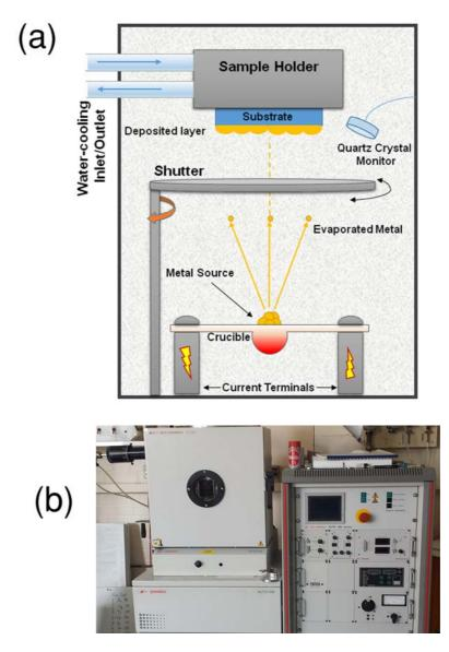
Figure 3.11: (a) Schematic Diagram of a Thermal Evaporator System and the (b) BOC Edwards Auto 500 Evaporator system
