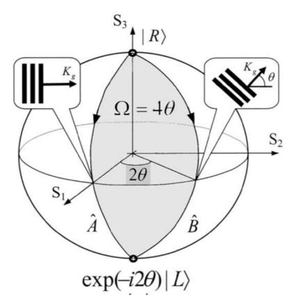
Figure 2.8: Representation of Geometric (Pancharatnam) phase introduced for space-varying angled elements [64]
