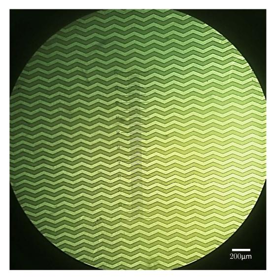
Figure 3.13: Photograph taken performing Optical microscopy of the herringbone pattern on a photomask
