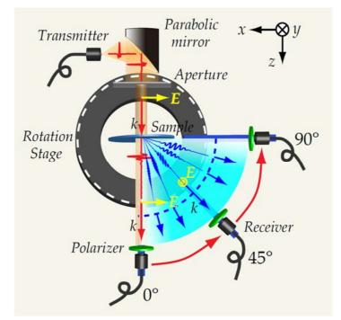
Figure 3.17: Schematic diagram of a THz-TDS experimental setup (Image from [83])
