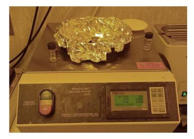
Figure 3.3: Close-up view of the Spincoater<sup>TM</sup> P6700 system
