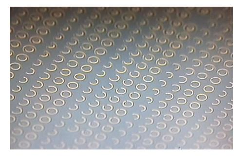
Figure 3.12: Optical Microscopy image of gold SRR's fabricated using lift-off process
