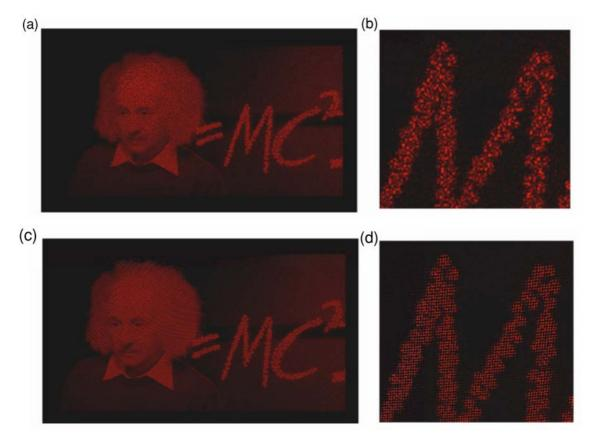
Figure B.3: Simulated Far-field images when using either a single or  $2 \times 2$  hologram array [67]
