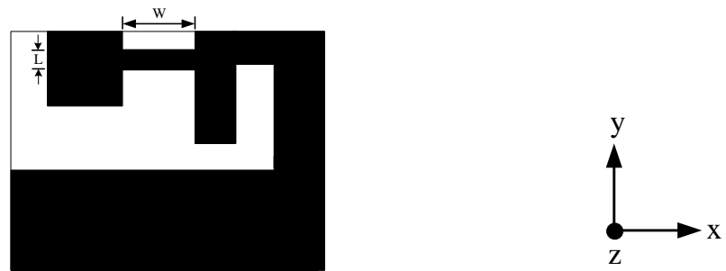
Figure 5.10: Dimensions of PIFA with 5 \times 1 \text{ mm}^2 copper bridge
