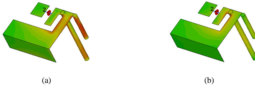
Figure 3.21: Current distribution of reconfigurable PIFA with PIN diode in OFF state at; (a) 2.01 GHz (b) 5.16 GHz
