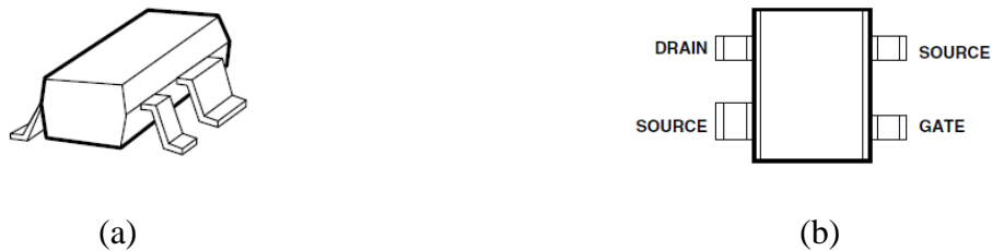
Figure 4.4: ATF 54143 E-PHEMT; (a) Surface mount package (b) Pin connections and package marking
