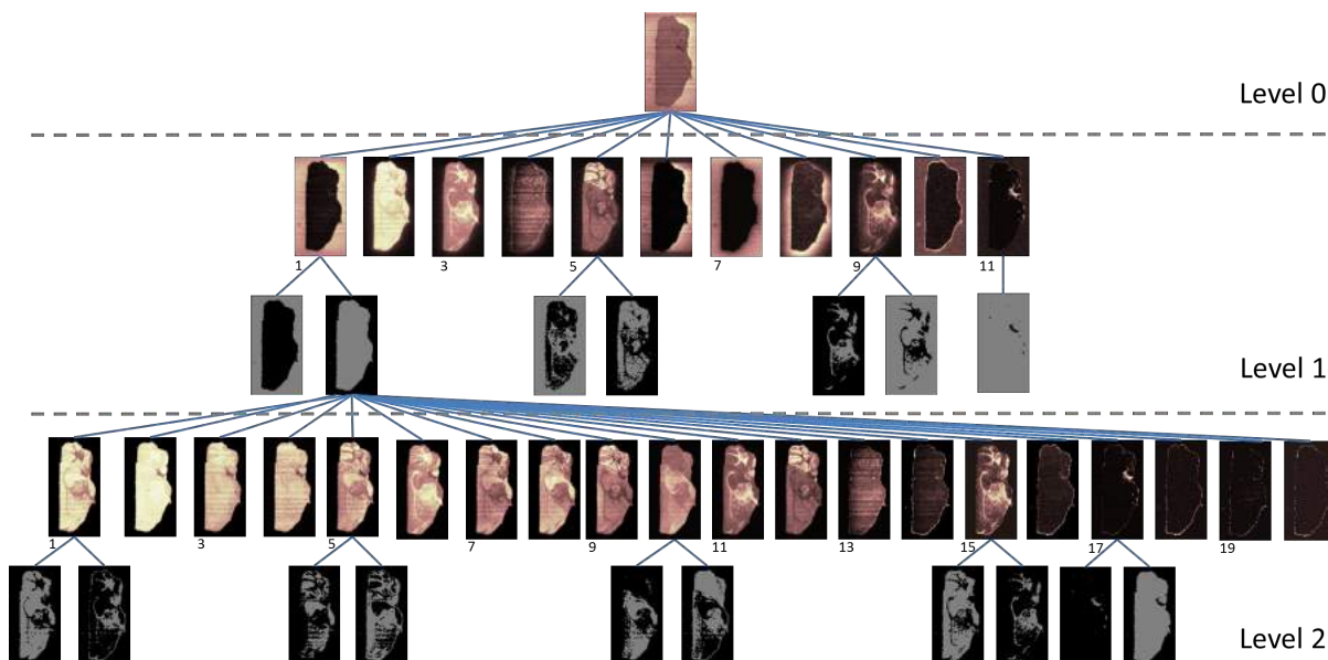
Figure 4.2: First 3 levels of the hierarchy generated using Algorithm 4.1. Masks used to split the data shown in grey. Mean ion image of each group shown at each level of the hierarchy.
