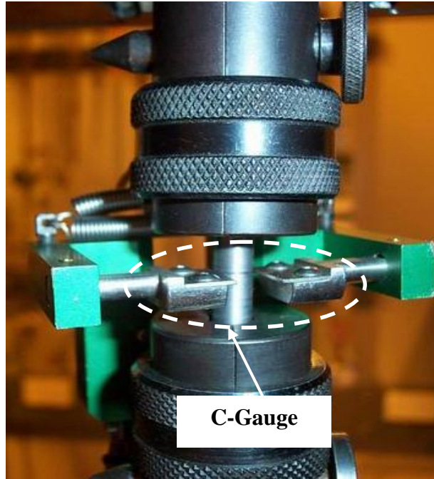
Fig. 4.3. C-strain transverse (diameter) extensometer.
