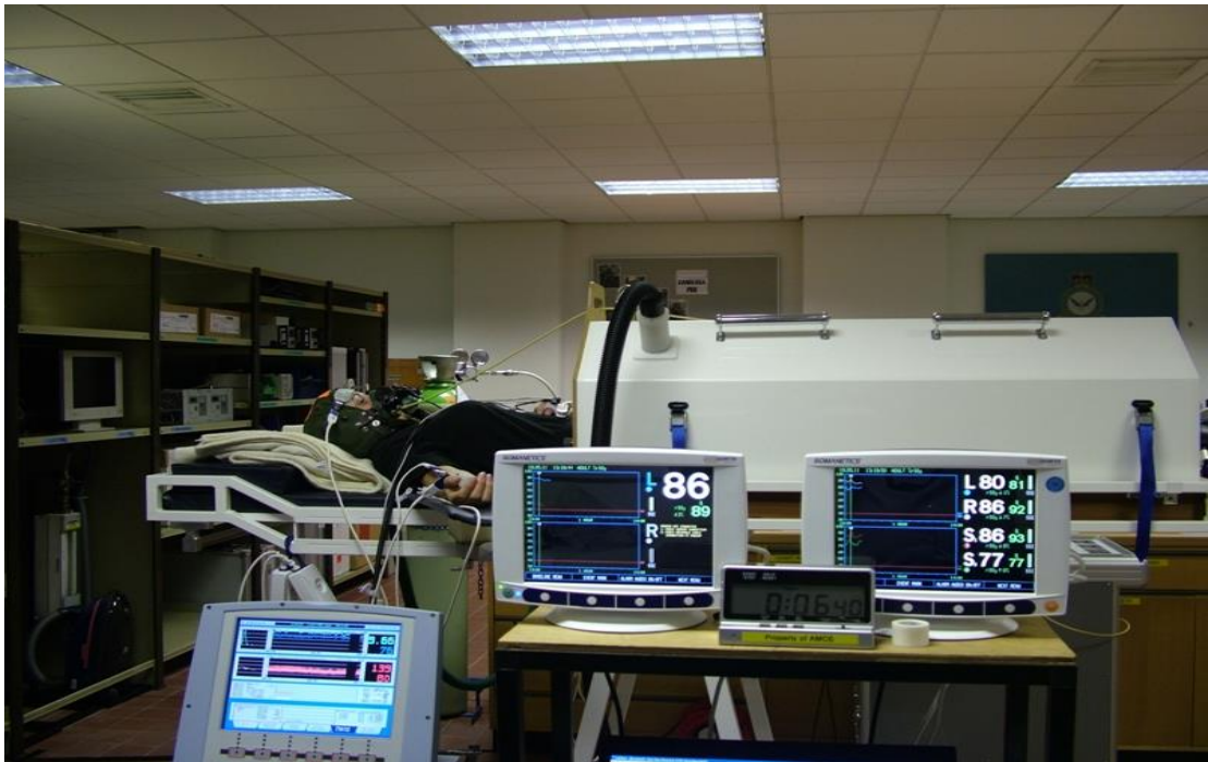
Figure 14. Study volunteer undergoing lower body negative pressure test in conjunction with the hypoxia altitude simulation test
